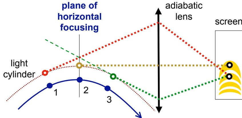
**Figure 3.** Optical device reproducing the hybrid impact parameter distribution of SR or LEBF on a screen. For the horizontal (resp. vertical) coordinate, the adiabatic lens is focused on the  $z = 0$  (resp.  $-\infty$ ) plane (the “vertical” axis  $\hat{y}$  is out of the figure plane). The hollow dots on the light cylinder are the classical emission points when the electron is in positions 1, 2 and 3. Rays emitted in 1 and 3 reach the same point on the screen, therefore interfere.
