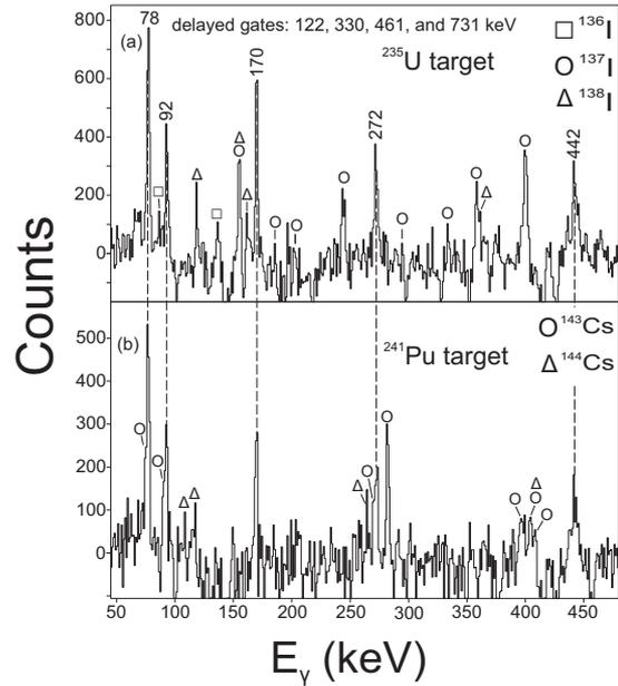
Fig. 3: Spectra of  $\gamma$ -rays prompt with fission events, obtained by summing double coincidence gates placed on all pairs of 122, 330, 461, and 731 keV delayed transitions. The panels refer to: (a) data taken with the  $^{235}\text{U}$  target; (b) with the  $^{241}\text{Pu}$  target. Transitions preceding the new 201 ns isomer are seen. The negative counts on both spectra result from the background subtraction.
