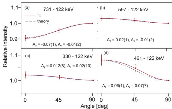
Fig. 4: (Color online) Selected examples of angular correlations in  $^{96}\text{Y}$ . The analysis was performed considering  $0^\circ$ ,  $45^\circ$ , and  $90^\circ$  (with  $135^\circ$  and  $180^\circ$  corresponding to  $45^\circ$  and  $0^\circ$ , respectively) average angles between the detectors, as done in refs. [26,27]. The energies of the  $\gamma$  transitions considered in each pair (see fig. 1) and the resulting  $A_2$  and  $A_4$  angular correlation coefficients are given.
