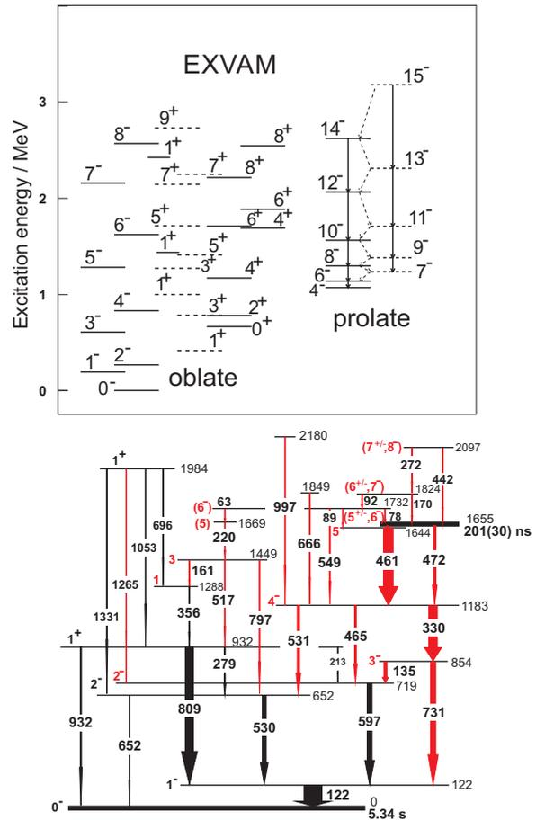
Fig. 1: (Color online) Experimental level scheme of  $^{96}\text{Y}$ : in black, transitions known prior to this work; in red, newly found transitions. The arrow widths reflect the observed transition intensities. Inset: theoretical spectrum obtained from the EXVAM model. The states are grouped according to the dominant oblate and prolate intrinsic quadrupole deformation.
