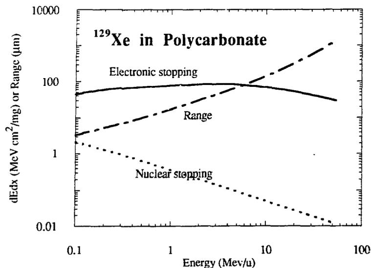
Fig. 4 - Stopping powers  $dE/dx$  ( $\text{MeV cm}^2/\text{mg}$ ) and Range ( $\mu\text{m}$ ) of  $^{129}\text{Xe}$  in polycarbonate as a function of beam energy ( $\text{MeV/u}$ ).
