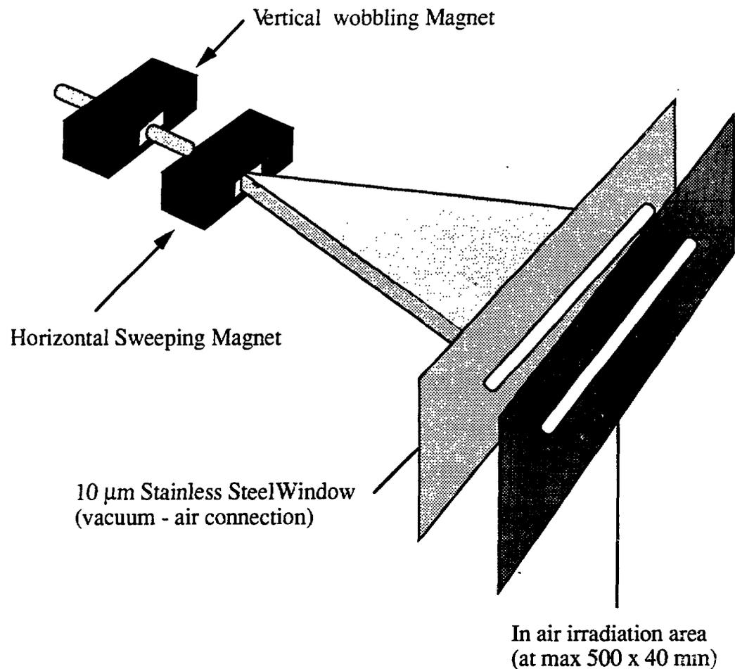
Fig. 2 - Schematic layout of the G4 beam line.
