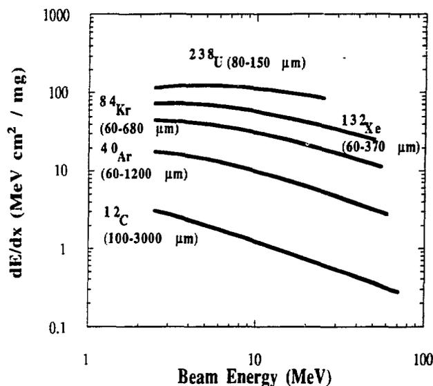
Fig. 5 -Domain of  $dE/dx$  as a function of incident energy illustrated for five different projectiles. For each ion, the ion range in Si for the two extreme available energies are given in parentheses.
