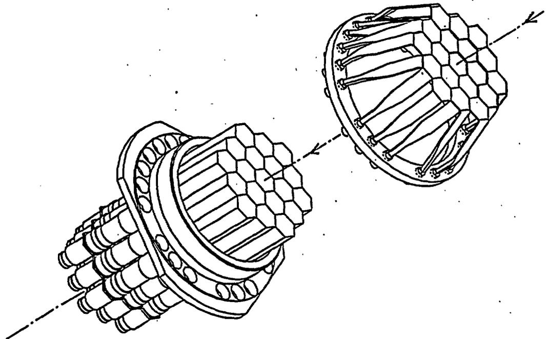
*Fig. 2 : The veto detector (upper right) and the associated module of 19 BaF<sub>2</sub> detectors (lower left) will be used to record  $\gamma$  signals and to discriminate against charged particules. The TAPS multidetector consists of 14 such modules.*
