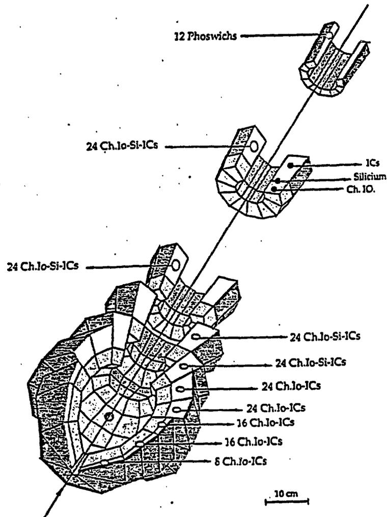
*Fig. 4 : A schematic view of the INDRA multidetector*
