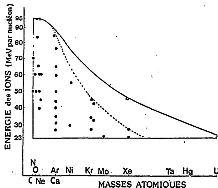
Xe ions be brought from 27 to 44 MeV per nucleon, but their intensity has increased typically from 50 nA to 800 nA.
