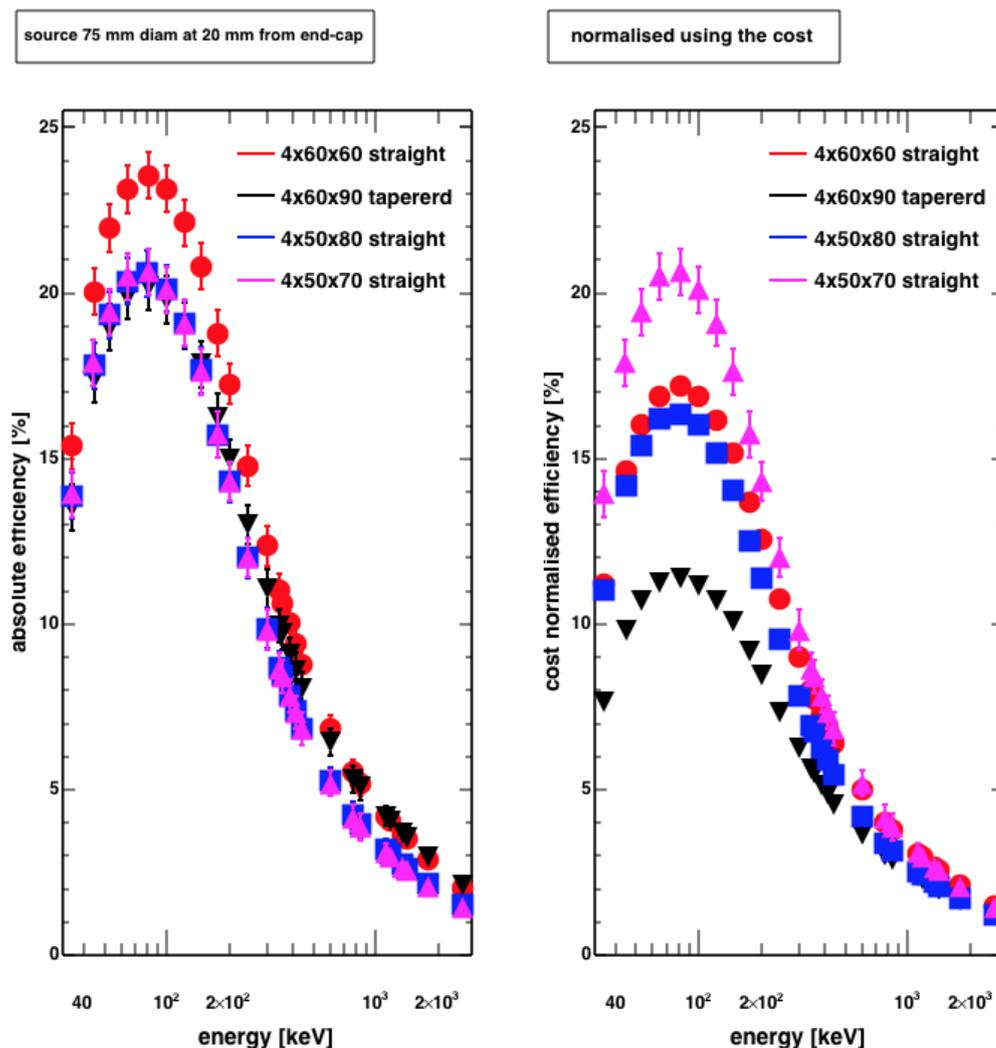
Figure 2: A comparison of the (left) absolute detection efficiencies and (right) cost-normalised absolute detection efficiencies for various clover detector geometries.
