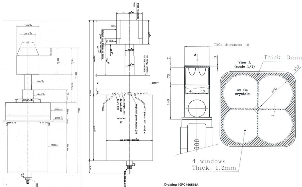
Figure 1: Schematic diagrams of some of the germanium detectors investigated. From left to right: a 469T BC (EXOGAM), a 466S BC, and a 457S.
