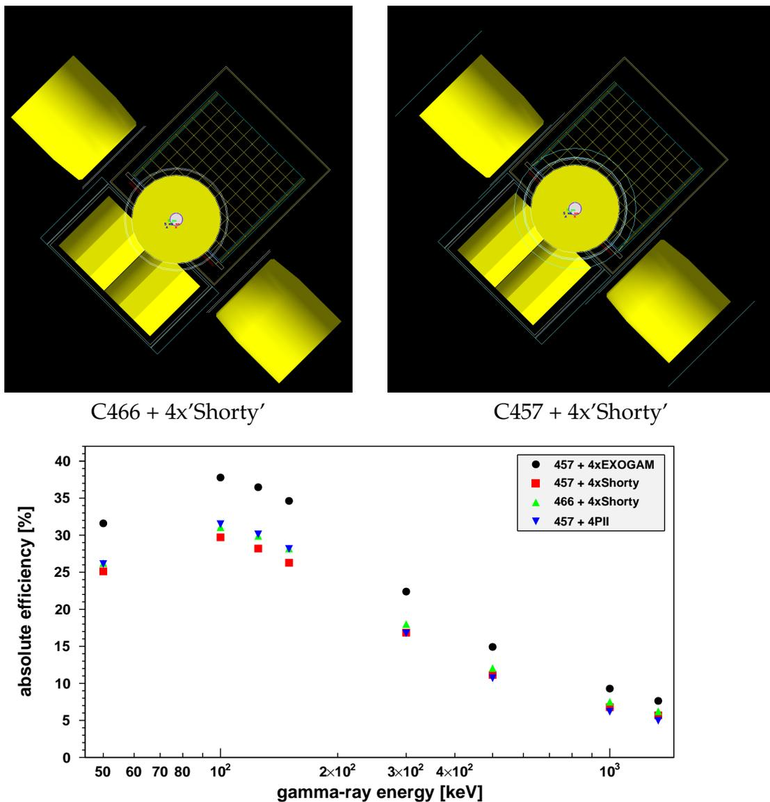
Figure 3: A comparison of the compact geometries possible with the (top-left) 466S and (top-right) 457S clover placed facing the DSSD. Bottom: absolute efficiency as a function of gamma-ray energy for various germanium detector combinations.
