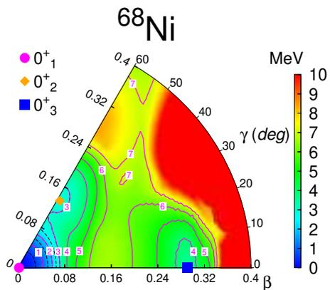
FIG. 10. (Color online) Potential Energy Surface from constrained Hartree-Fock minimization in the shell-model basis for  $^{68}\text{Ni}$ . The three predicted  $0^+$  minima of the PES, spherical, oblate and prolate, are shown with different symbols.
