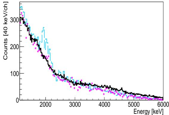
FIG. 7. (Color online) Comparison between the experimental Doppler-corrected energy spectrum for a  $^{68}\text{Ni}$  beam on a C target (solid black histogram) and simulated spectra assuming  $\beta_N = 0.1$  (magenta stars) and  $\beta_N = 0.2$  (dashed blue histogram). The adopted value of  $\beta_N = 0.102(8)$ , as deduced from the study with the Pb target, is too small for a peak to be seen when  $^{68}\text{Ni}$  scatters off the C target.
