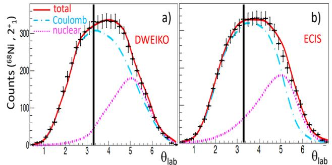
FIG. 6. (Color online) Same as Fig. 3 but for  $^{68}\text{Ni}$ .  $B(E2; 0_{g.s.}^+ \rightarrow 2_1^+)$  values of 292(35) and 312(40)  $e^2\text{fm}^4$  are obtained from the comparison between the experimental distribution (black crosses) with the DWEIKO (a) and ECIS (b) codes, respectively.
