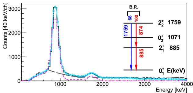
FIG. 2. (Color online) Doppler-corrected and background-subtracted  $\gamma$ -ray spectrum of  $^{70}\text{Zn}$  measured with Château de Cristal (black histogram). The intensities of the two peaks were determined using the simulated response function of the array (dashed magenta line) on top of two exponential functions accounting for the background (long-dashed gray line). The result of the best fit procedure is illustrated with blue circles.
