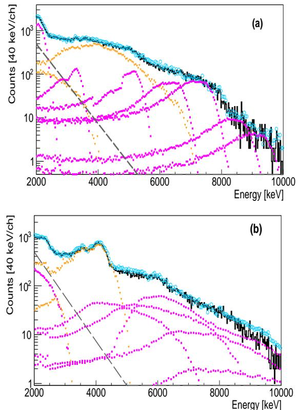
FIG. 8. (Color online) (a): Doppler-corrected experimental  $\gamma$ -ray spectra of  $^{68}\text{Ni}$  (black histogram) compared to GEANT4 simulations (open blue circles) including the excitation of several in-flight  $\gamma$ -ray components (magenta squares) discussed in the text and the excitation of the  $2_1^+$  and  $3_1^-$  states of the  $^{208}\text{Pb}$  target (orange triangles). (b): same as (a) but non Doppler-corrected.
