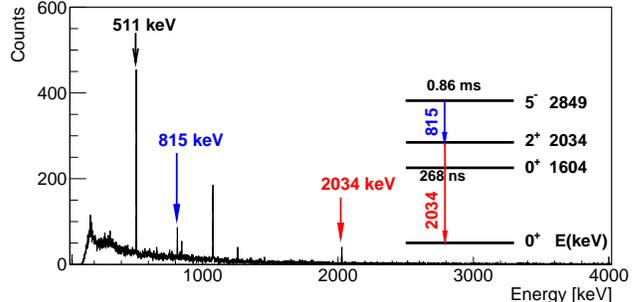
FIG. 1. (Color online)  $\gamma$ -ray spectrum of one HPGe detector associated with the de-excitation of  $^{68}\text{Ni}$  implanted in the plastic detector. The lines corresponding to the decays of the  $0_2^+$  and  $5^-$  isomers are indicated by arrows.
