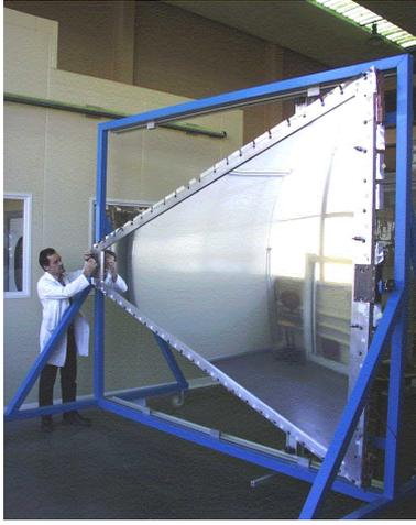
Figure 36: One MDC-IV in construction at IPN Orsay
