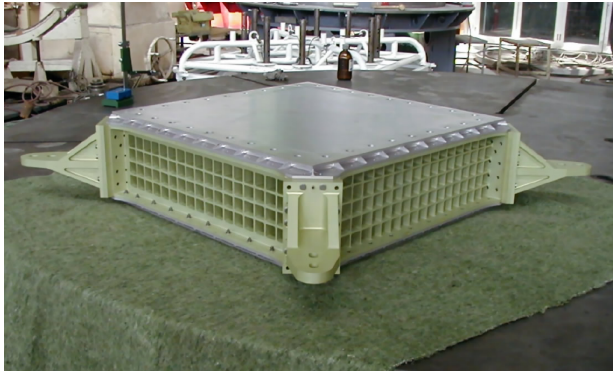
Figure 1. ECAL for the AMS-02 experiment inside the supporting structure. 324 photomultipliers will be housed in the lateral panels. The electromagnetic shower is sampled in X and Y directions by scintillating fibers glued to the inside of the grooved lead foils.
