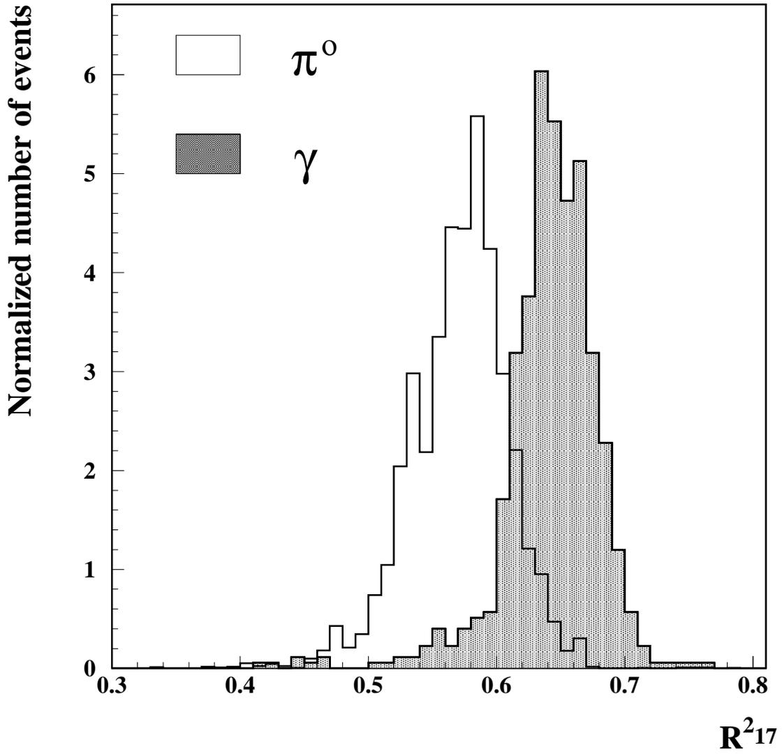
Figure 23: Distribution of dispersion ratio ( $R_{17}^2$ ) for  $\gamma$  and  $\pi^0$  of  $E_t=50$  GeV and at  $\eta=0.67$
