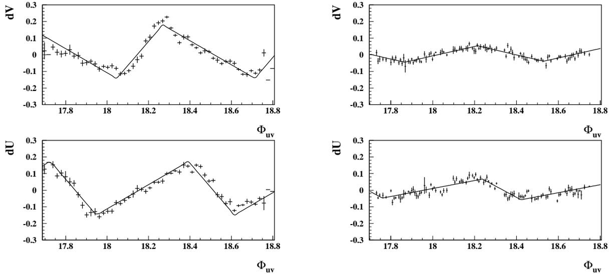
Figure 16:  $w - w_{beam}$  vs  $\phi_{uv}$  ( $w=u$  or  $v$ ) after correction of the function of figure 15 (points with error bars).  $\phi_{uv}$  is given here in cell units of the middle sampling. Left histograms are data and right ones are Monte-Carlo.
