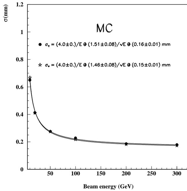
Figure 18: Position resolution for sampling UV
