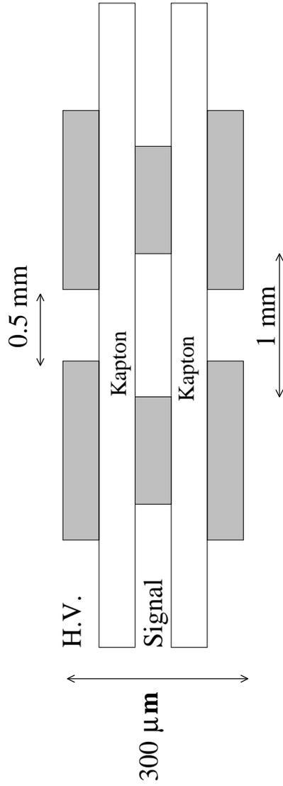
Figure 4: Transverse cut of an electrode (the grey areas are the copper pads).
