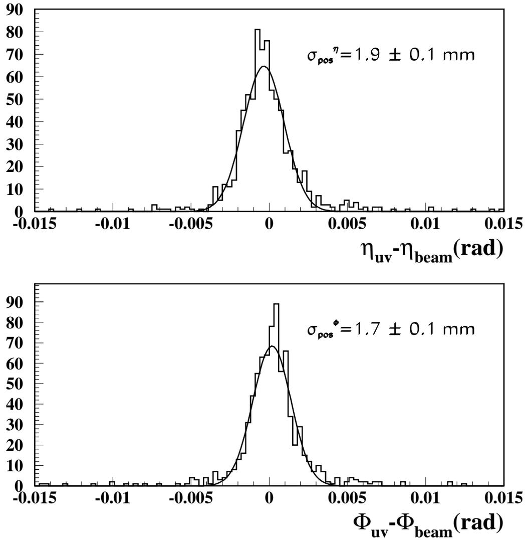
Figure 6: Resolution in position for muons in the UV sampling.
