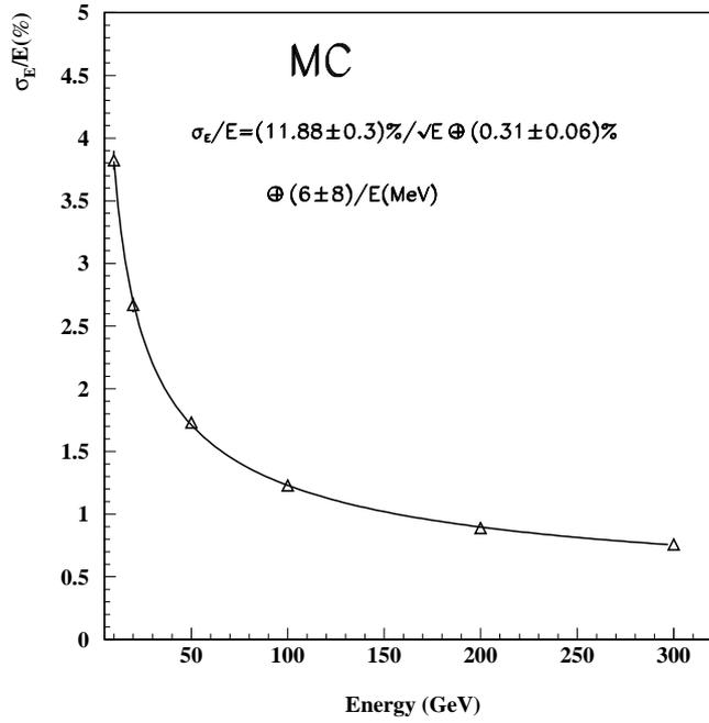
Figure 12: Energy resolution as a function of energy (GaAs). For the data, the noise contribution was fixed to the measured values with random triggers (356 MeV); for the simulation, it was fitted and found compatible with zero as expected.
