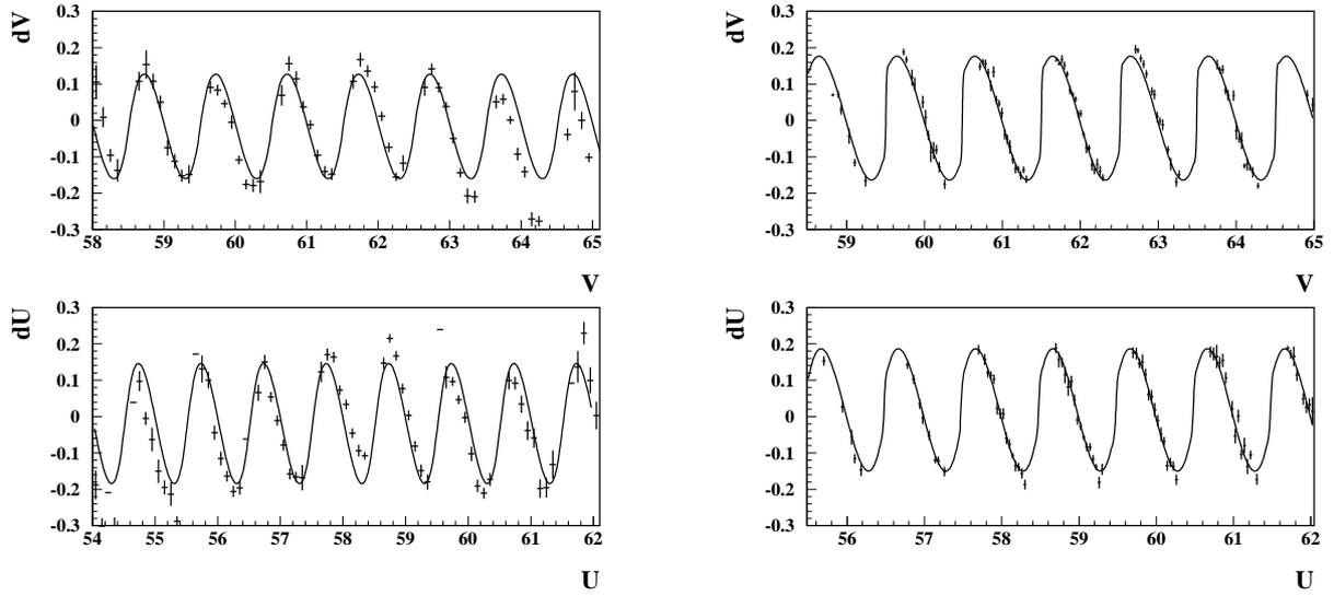
Figure 15:  $w - w_{beam}$  vs  $w$  ( $w=u$  or  $v$ ) before any correction (crosses), and correction function (full line). Numbers are in  $U$  and  $V$  cell units. Left histograms are data and right ones are Monte-Carlo.
