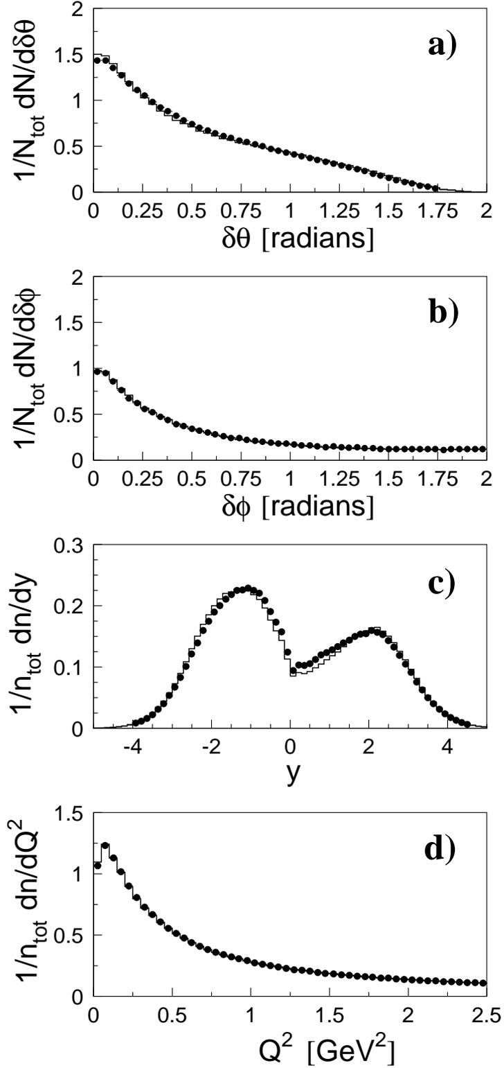
Figure 1: Distributions of (a) the difference in polar angle of pairs of tracks,  $\delta\theta$ , (b) the difference in azimuthal angle of pairs of tracks,  $\delta\phi$ , (c) the single-particle rapidity with respect to the thrust axis,  $y$ , and (d) the inclusive four-momentum difference squared,  $Q^2$ , for uncorrected data (points) compared to the predictions of JETSET after detector simulation (histogram).
