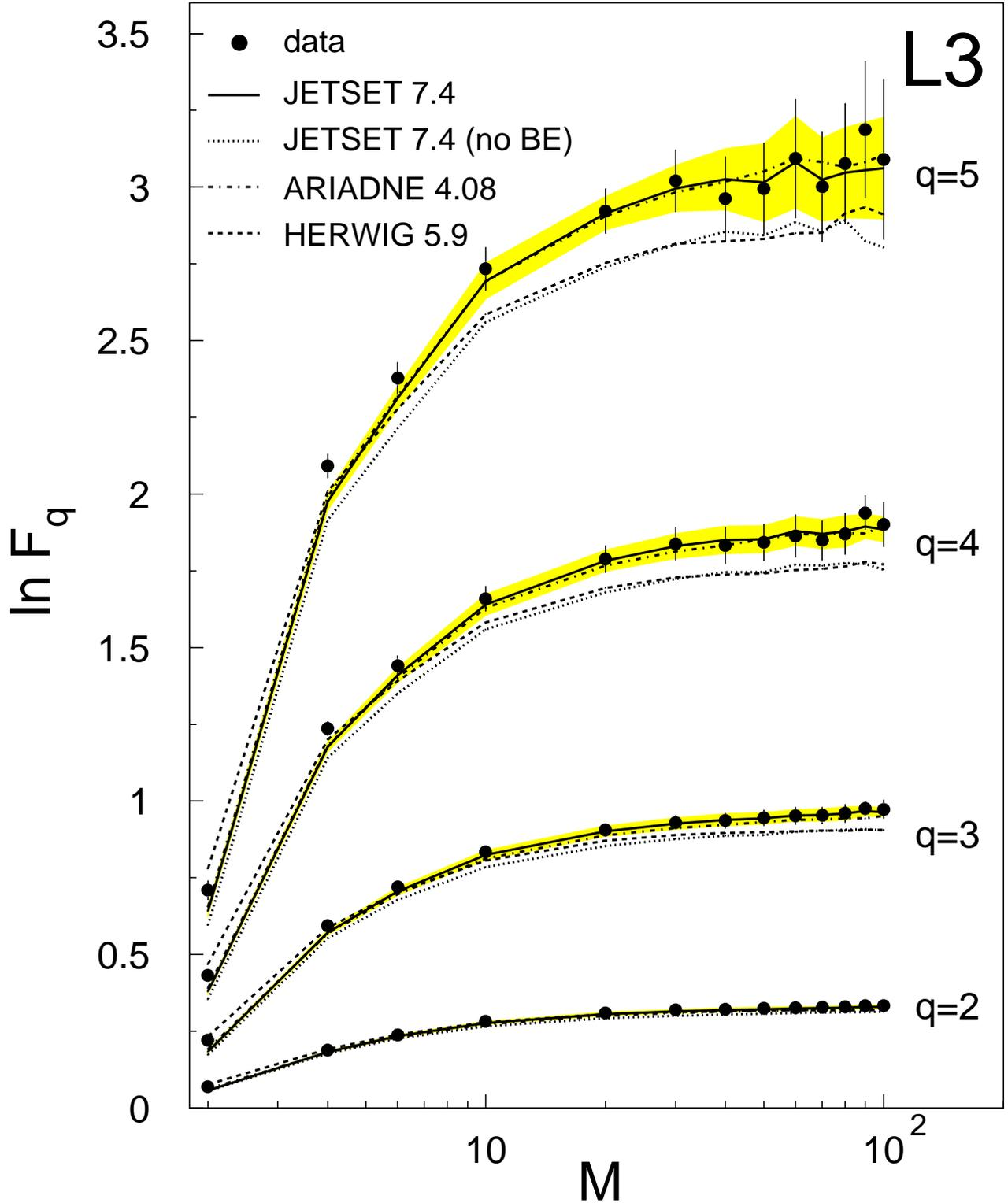
Figure 2: NFMs as a function of the number of bins,  $M$ , in the transformed rapidity defined with respect to the thrust axis. In this and the following figures the shaded areas represent the errors on the JETSET predictions. The errors on the ARIADNE predictions are comparable whereas those on the HERWIG predictions are about 50% larger.
