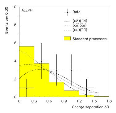
Figure 17: Distribution of the charge separation  $\Delta Q$  for the 12 peak events (triangle with error bars), and as predicted from standard processes (shaded histogram). The predictions of particle pair production with subsequent decays into udud (dotted curve)  $c\bar{s}\bar{c}s$  (dash-dotted curve) and  $uu\bar{u}\bar{u}$  (dashed curve) are also indicated.
