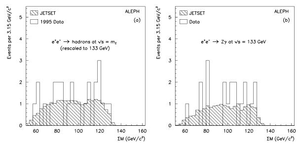
Figure 5: Distribution of the sum of the di-jet masses for the combination with the smallest mass difference (a) for the 1995 data collected at the Z peak just prior to the high energy run (the total energy is rescaled to 133 GeV); and (b) for the  $e^+e^- \rightarrow Z\gamma$  events collected during the high energy run. The hatched histograms are the distributions expected from JETSET.
