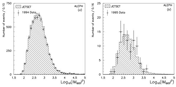
Figure 8: Distribution of the QCD matrix element squared for four-jet events (a) in 1994 and (b) in 1995 prior to the high energy run. The hatched histogram is the prediction from JETSET.
