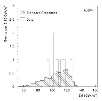
Figure 6: Distribution of the di-jet mass sum for the combination with the second-smallest mass difference in the data, once the nine events around 105  $\text{GeV}/c^2$  are removed. The hatched histogram is the distribution expected from the simulation of the standard processes, obtained with the same procedure and normalized to seven events.
