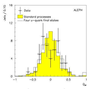
Figure 19: Jet charge distribution (four entries per event) for the 12 peak events (triangles with error bars), for a normal mixture of standard four-jet events (shaded histogram) and for uūuū events (dashed histogram). The histograms are normalized to 12 events.
