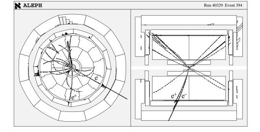
Figure 3: Candidate four-fermion  $e^+e^-q\bar{q}$  event. In this event display, the central region has been expanded to emphasize the tracking detectors.
