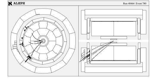
Figure 4: Candidate four-fermion  $\nu \bar{\nu} q \bar{q}$  event. In this event display, the central region has been expanded to emphasize the tracking detectors.
