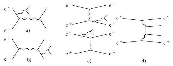
Figure 1: Feynman diagrams for four-fermion final states involving only  $\gamma$  or Z exchange: a) conversion, b) annihilation, c) Bremsstrahlung, d) multiperipheral. The wiggly lines represent a  $\gamma$  or a Z exchange. The solid lines not labelled as  $e^{\pm}$  may be quarks or leptons.
