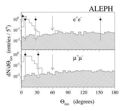
Figure 2: The lepton pair isolation,  $\Theta_{iso}$ , for  $e^+e^-q\bar{q}$  and  $\mu^+\mu^-q\bar{q}$  candidates after all cuts (except isolation) have been applied. Presented are the expectations from FERMISV (hatched), the background (mostly  $q\bar{q}$ , solid) and the data (dots). The histograms are normalized to the expectations in 5.8 pb<sup>-1</sup> of data. The cut  $\Theta_{iso} > 60^{\circ}$  is indicated with an arrow.
