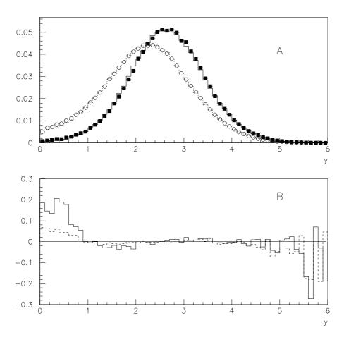
Figure 3: A) Rapidity distributions of Monte Carlo (dashed line) and data (hollow circles) for Normal cuts and of Monte Carlo (solid line) and data (black squares) for High momentum cuts. B) Normalized differences (Monte Carlo - Data)/(Monte Carlo + Data) for Normal (dashed line) and High momentum (solid line) cuts.
