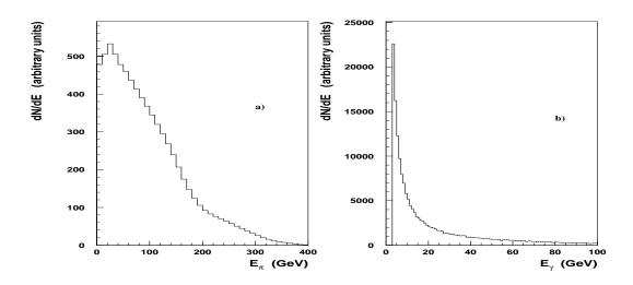
Fig. 2. a) The energy spectrum of  $\pi^0$ 's produced in 450 GeV proton collisions with the neutrino target in a cone of  $\sim 2 \text{ mrad. } b$ ) Energy spectrum of the photons crossing the horn magnetic field and momenta pointing towards the NOMAD fiducial area.
