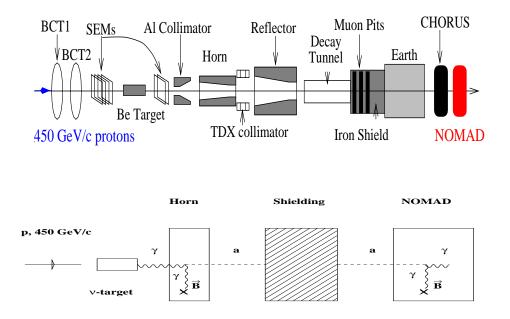
Fig. 1. Schematic layout of the WANF beam line (not to scale) and an illustration of the principle of the WANF-NOMAD high energy photon-regeneration experiment.
