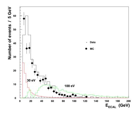
Fig. 4. The ECAL energy spectra for candidate (solid line) and background (full circles) events. Systematic errors are not shown. The shape of the axion signals corresponding to masses  $m_a = 30 \text{ eV}$  and  $m_a = 100 \text{ eV}$  are shown for comparison.
