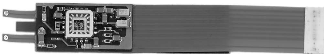
figure 2: multilayer board with kapton flex assembling
