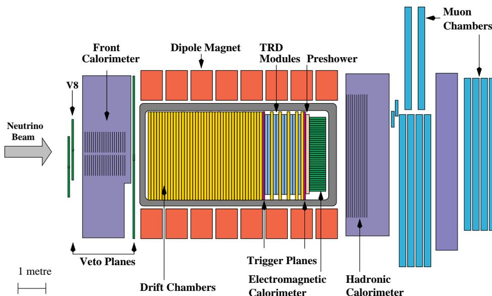
Figure 1: Side view of the NOMAD detector. The coordinate system has the  $x$ -axis into the plane of the figure, the  $y$ -axis directed up towards the top of the figure and the  $z$ -axis horizontal, approximately along the direction of the neutrino beam (which points upwards at an angle of  $2.4^\circ$  with respect to the  $z$ -axis).
