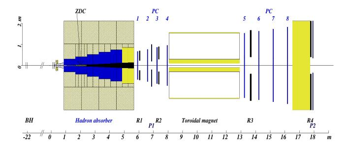
Fig. 1. The NA50 apparatus. Details of the target area are shown in figure 2.
