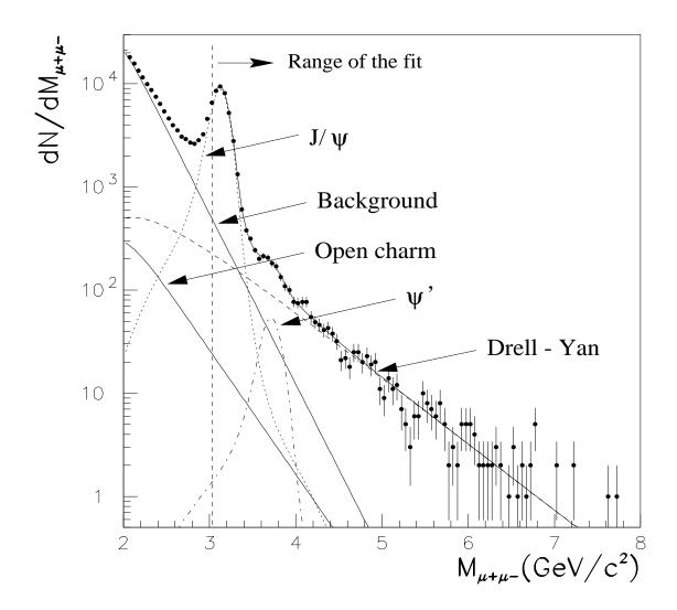
Fig. 3. Muon pair invariant mass spectrum for Pb-Pb collisions at  $158~{
