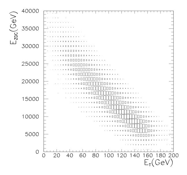
Fig. 5. Observed correlation between the neutral transverse energy measured in the electromagnetic calorimeter and the forward energy measured by the "zero degree calorimeter". The data correspond to dimuon events with  $M_{\mu\mu}>2.0~{\rm GeV}/c^2$ , not corrected for subtarget identification efficiency.
