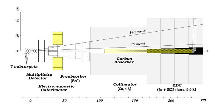
Fig. 2. Lay-out of the various elements of the NA50 detector in the target area.
