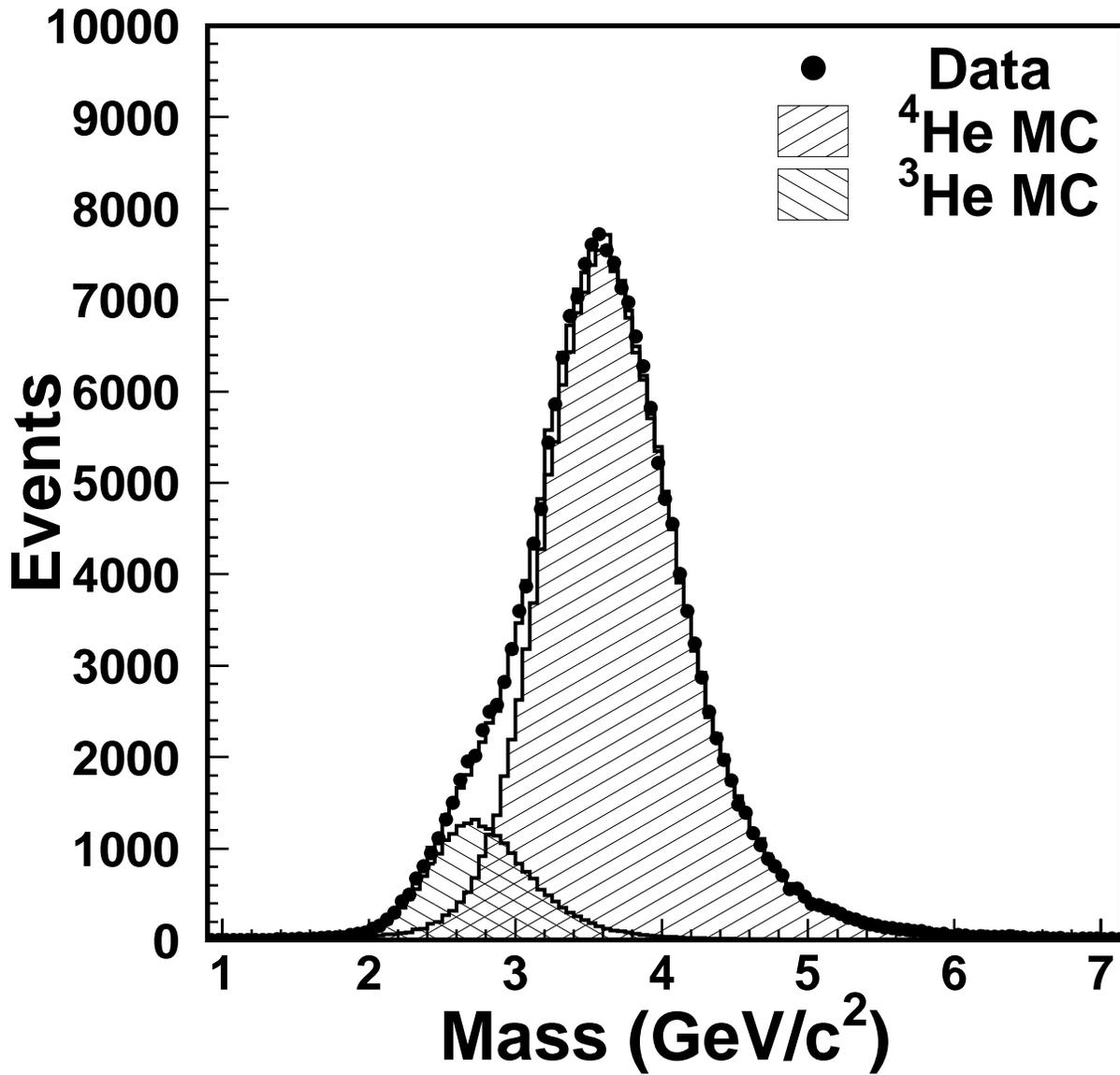
Figure 4: Mass distribution for helium events above geomagnetic cutoff for  $|\Theta_M| > 0.9$  and  $\beta < 0.9$ . Filled circles are data for period (c). Histogram is a Monte Carlo simulation with 11.5%  $^3\text{He}$ .
