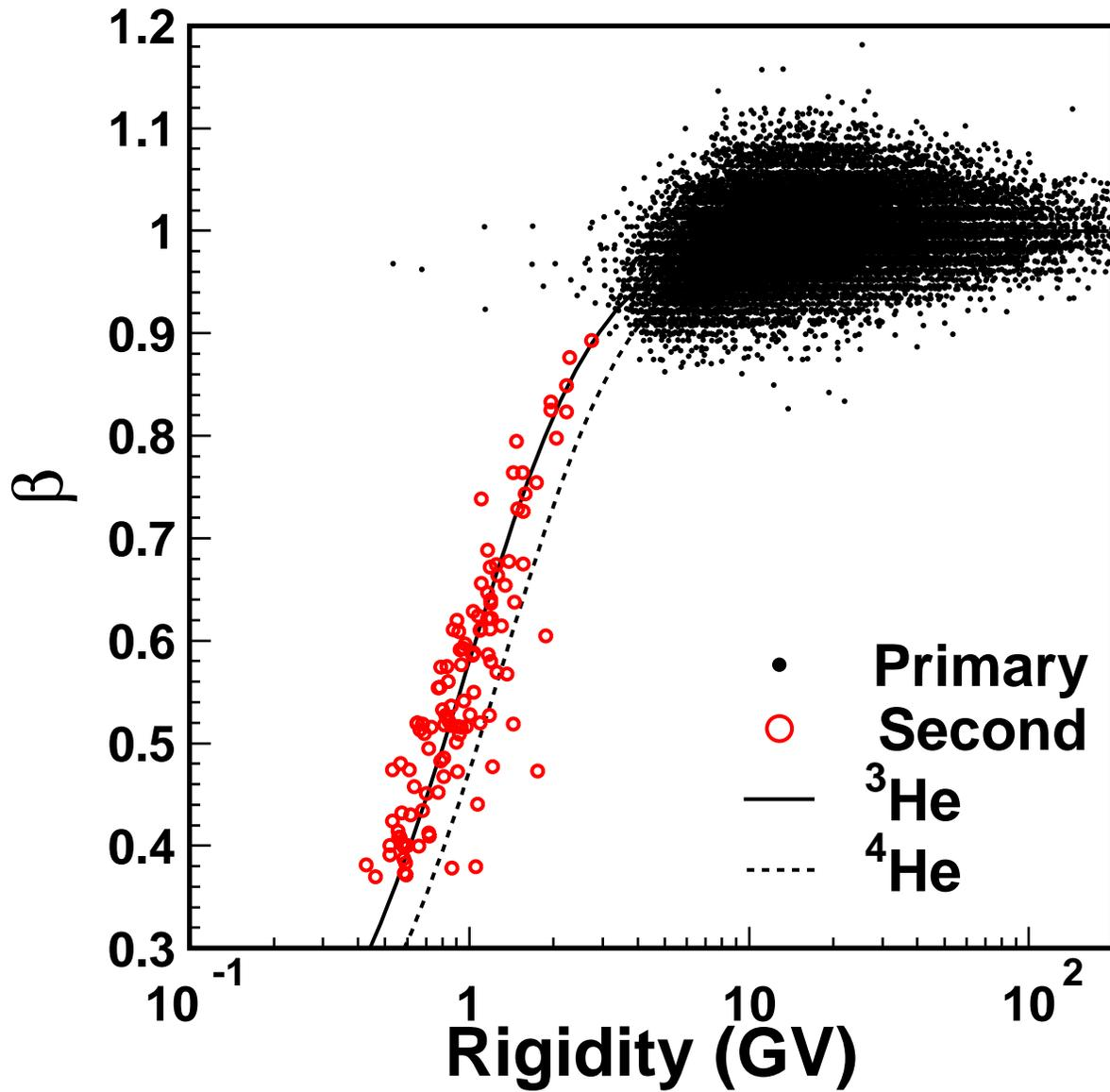
Figure 5: Correlation between rigidity and velocity for helium events detected at  $|\Theta_M| < 0.6$ . Dots denote events from the primary spectrum, and open circles those from under cutoff. The solid (dashed) line corresponds to  ${}^3\text{He}$  ( ${}^4\text{He}$ ).
