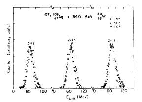
Fig. 14 : Width of the quasi-fission fragment kinetic energies. The kinetic energy distribution has been measured for several fragments at different angles in the system ( $^{40}$ Ar +  $^{107}$ ,  $^{109}$ Ag)(ref. 24).
