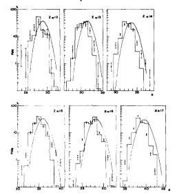
Fig. 31.a : Mass distribution for fixed  $\_$  values in the products of the reaction  $({}^{40}\text{Ar} + {}^{238}\text{U})$ . The continuous curve represents the calculation according equations (32) and (33). The histogramm is obtained after correcting for neutron evaporation (ref. 54).
