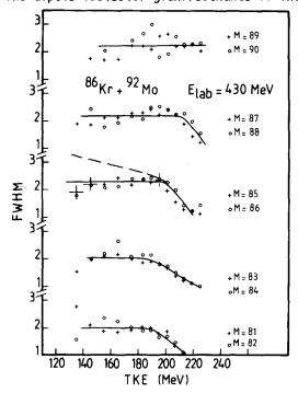
Fig. 30 : Z distribution width for fixed mass number versus total kinetic energy loss for deep inelastic products obtained in the reaction ( $^{86}$ Kr +  $^{92}$ Mo). The dotted line expresses what would be a temperature depandent correlation in the case of A = 86 ( $\Gamma \propto \sqrt{T/C}$ ) (ref. 52).
