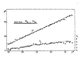
Fig. 34 : Number of missing mass units,  $v_n$ , versus Z of the fragments in deep inelastic reactions induced by  $4^{0}$ Ar on Ag targets, deduced by difference between measured masses and the mass of the composite system (after correction of 1.3 charge units) (ref. 69).
