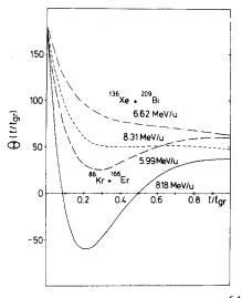
Fig. 24 : Theoretical calculations 61 for mean deflection functions of several systems, obtained by coupling to the  $\Delta\theta$  equation (39) the kinetic energy equation (41). Systems ( $^{86}$ Kr +  $^{166}$ Er) and ( $^{136}$ Xe +  $^{209}$ Bi) at two bombarding energies.
