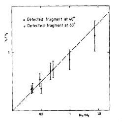
Fig. 38 : Ratio  $v_1/v_2$  of the number of neutrons associated with each fragment 1 and 2, versus their mass ratio  $M_1/M_2$ .
