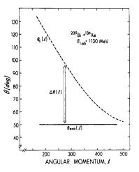
Fig. 23 : Difference between the coulomb deflection function and the deep inelastic deflection function (system  $^{136}Xe + ^{209}Bi$ ) (ref. 60).
