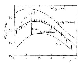
Fig. 8.a : Mean kinetic energies for the fully relaxed events (quasi-fission) of various Z. Dotted line : calculated energies assuming  $E_{\rm COU1} + E_{\ell}$  for two bombarding energies : 182 and 280 MeV for the system (<sup>40</sup>Ca + <sup>6</sup> \*Ni). Full points : experimental results at 182 MeV. Stars : experimental results at 280 MeV (ref. 22).
