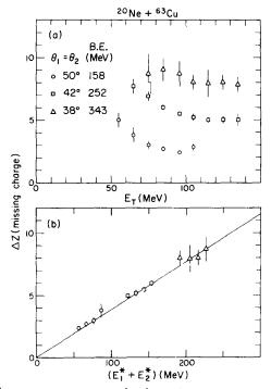
$\underline{Fig. 32}$  : a- Mean missing charge versus  $E_T$  for three different bombarding energies.
