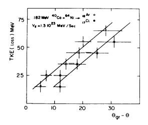
Fig. 28 : Variation of the mean total kinetic energy loss versus rotation angle of the composite system ( ${}^{40}Ca + {}^{64}Ni$ ) for the products Z = 17 and Z = 18 (ref. 22).
