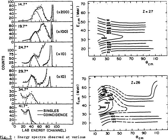
Fig. 9 : Energy spectra observed at various angles for krypton-like fragments in the
