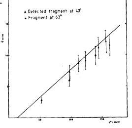
Fig. 39 : Total neutron multiplicity  $v_T$  as a function of the excitation energy of both fragments. The line is obtained in a calculation assuming statistical theory. For  $v_T = 0$  the excitation energy is due to gamma ray emission (ref. 72).
