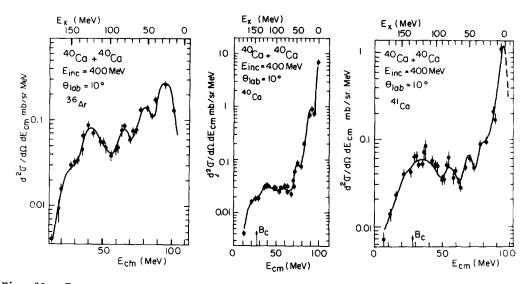
Fig. 29 : Energy spectra for several fragments close to the projectile <sup>40</sup>Ca, in the deep inelastic events produced in the reaction (<sup>40</sup>Ca + <sup>40</sup>Ca) at 400 MeV. Well marked bumps appear at 30 and 55 MeV (ref. 49).
