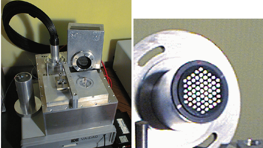
Figure 2: Left: HPD test setup in Lyon. The HPD is inside the metallic box. The clear fiber bundle is visible on top of this box. Also shown is the VA-DACQ acquisition system from IDEAS for the VA-TA readout. Right: details of the HPD cookie collecting fibers at the HPD entrance window. The hexagonal pattern matches the HPD pixel distribution.
