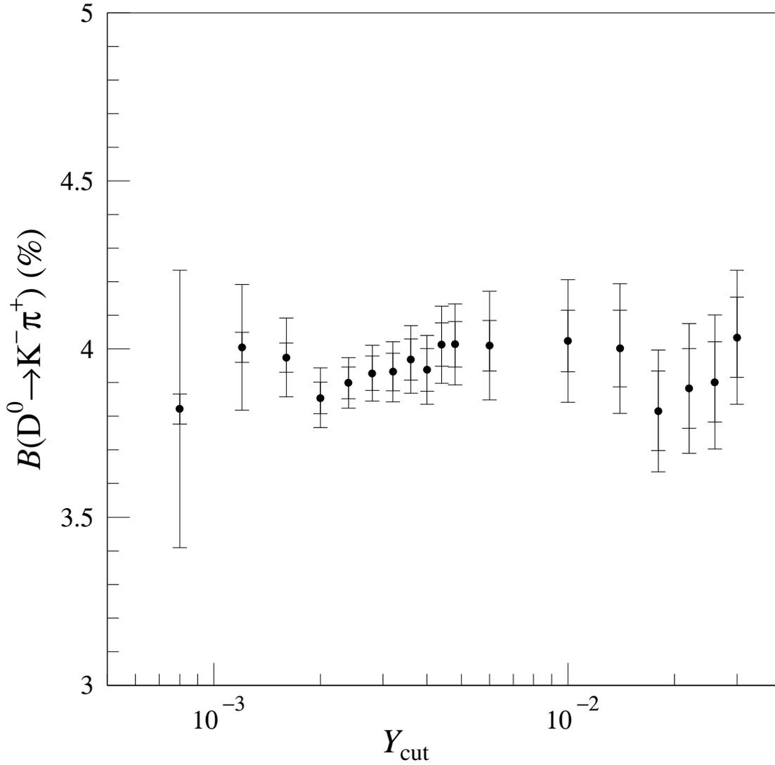
Figure 4: Measurements of  $B(D^0 \rightarrow K^- \pi^+)$  as a function of the jet mass parameter  $Y_{\text{cut}}$ . The large error bars represent the total uncertainty, while the smaller ones indicate the statistical component of the error. The result for  $Y_{\text{cut}} = 0.0024$  has minimal total error.
