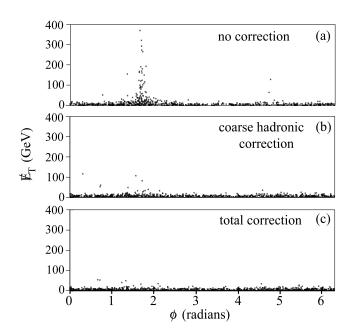
FIG. 36. Effect of Main-Ring  $E_T^{\rm cal}$  corrections:  $E_T^{\rm cal}$  vs  $\phi$  for MRBS events for (a) no correction, (b) CH correction, and (c) total correction.
