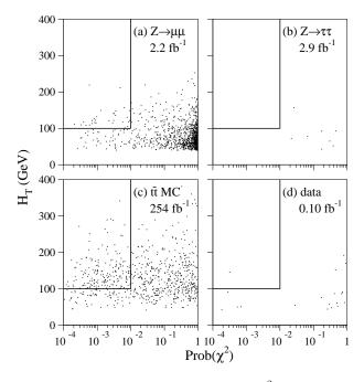
FIG. 12. Scatter plots of  $H_T$  vs  $\operatorname{Prob}(\chi^2)$  for the  $\mu\mu$  channel: (a)  $Z \to \mu\mu$  background, (b)  $Z \to \tau\tau \to \mu\mu$  background, (c)  $t\bar{t} \to \mu\mu$  signal, and (d) data. The signal region is shown in the upper left corner of each plot  $(\operatorname{Prob}(\chi^2) < 1\%, H_T > 100 \text{ GeV})$ .
