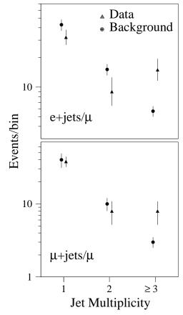
FIG. 26. Inclusive jet multiplicity spectra for  $\ell$ +jets/ $\mu$  data (circles) and expected background (triangles) obtained prior to applying the  $\mathcal A$  and  $H_T$  requirements. Note that good agreement is seen for the  $\geq 1$  and  $\geq 2$  jet bins, but the  $\geq 3$  jet bin shows a clear excess in the data.
