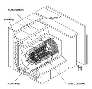
FIG. 7. Cutaway view of the D $\emptyset$  detector, showing the tracking chambers, calorimetry, and muon system.
