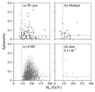
FIG. 27. Scatter plots of  $\mathcal{A}$  vs  $H_T$  for the  $e+\text{jets}/\mu$  channel for (a) VECBOS W+jets MC background, (b) QCD multijet background, (c) HERWIG  $t\bar{t}$  MC events  $(m_t=170~\text{GeV}/c^2)$ , and (d) data.
