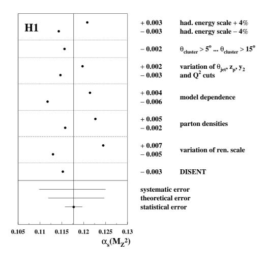
Figure 6: List of systematic uncertainties on the fitted value of  $\alpha_s$ . The horizontal lines separate different classes of uncertainties. The vertical line indicates the central value of  $\alpha_s(M_Z)$  resulting from the fit. The black points give the values of  $\alpha_s$  that are obtained when each source of systematic error is varied as described in the text. The uncertainties of the three classes below the dashed horizontal line are combined to give the theoretical error.
