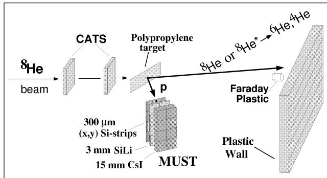
Figure 1. *Experimental set-up in the reaction chamber.*
