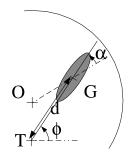
Fig. 1. Definition of geometrical parameters used for the shower reconstruction. O is the center of the camera, G the image barycenter and T the reconstructed target direction.
