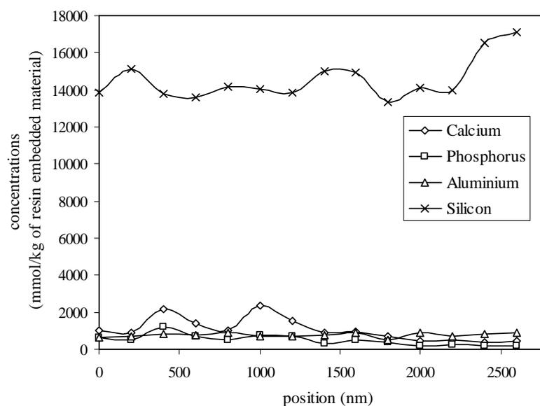
Figure 1 : Ca, P, Al and Si concentrations ( $\text{mmol.kg}^{-1}$  of resin embedded material) profiles across the periphery of bioactive glass particles at 1 day after immersion in a standard culture medium.
