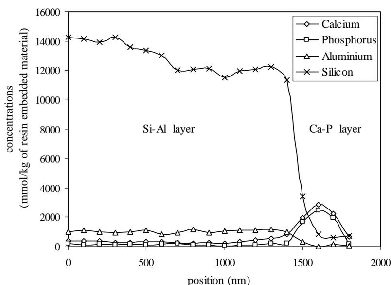
Figure 2 : Ca, P, Al and Si concentrations ( $\text{mmol.kg}^{-1}$  of resin embedded material) profiles across the periphery of bioactive glass particles at 2 days after immersion in a standard culture medium.
