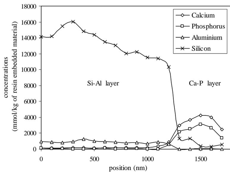
Figure 4 : Ca, P, Al and Si concentrations ( $\text{mmol.kg}^{-1}$  of resin embedded material) profiles across the periphery of bioactive glass particles at 4 days after immersion in a standard culture medium.
