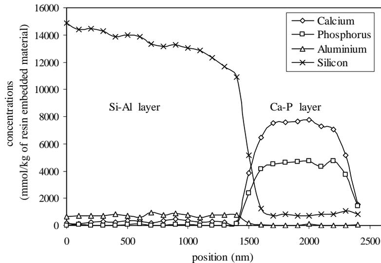
Figure 5 : Ca, P, Al and Si concentrations ( $\text{mmol.kg}^{-1}$  of resin embedded material) profiles across the periphery of bioactive glass particles at 28 days after immersion in a standard culture medium.
