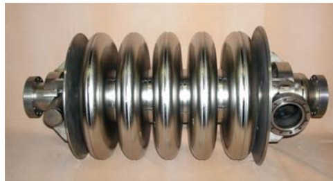
Fig. 8 700 MHz (beta 0.47) cavity (INFN-Milano)
