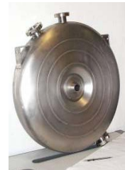
Fig. 5 Superconducting re-entrant structure (INFN-Legnaro)
