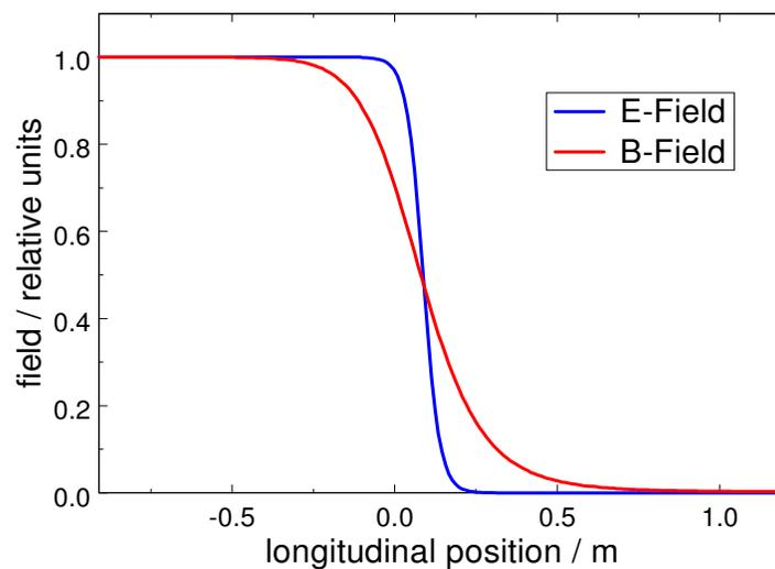
**Figure 7: Electric and magnetic fields along the axis at the LISE Wien filter exit as measured and modelled with the Enge model [6]. The mismatch between the electric and magnetic fringe field causes a resolution weakening.**
