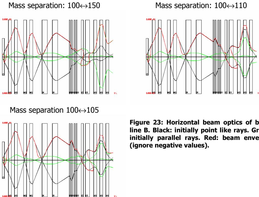
**Figure 23: Horizontal beam optics of beam line B. Black: initially point like rays. Green: initially parallel rays. Red: beam envelope (ignore negative values).**
