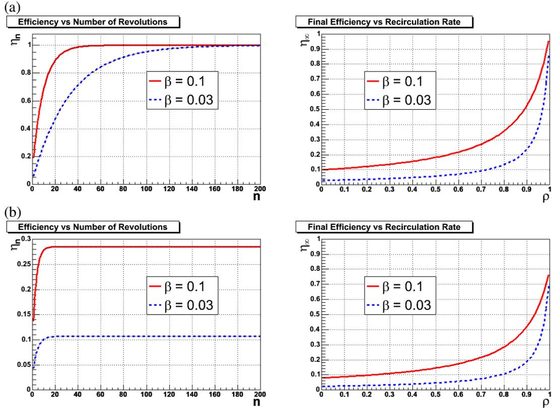
**Figure 28: Efficiencies of ion recirculation versus number of cycles (left) and recirculation rate (right) for (a) ideal values of recirculation and extraction rates  $\varepsilon = 1$  and  $\rho = 1$  and (b) realistic values  $\varepsilon = 0.8$  and  $\rho = 0.8$ .**
