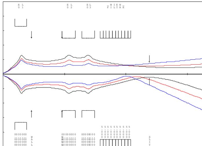
**Figure 17: Horizontal (below) and vertical (above) beam envelopes in the extraction line of a beam with  $A = 100$  (black curves),  $A = 40$  (red curves) and  $A = 16$  (blue curves) for an extraction voltage of  $U_{ext} = 60$  kV and a beam intensity of  $I = 2.0$  mA. The length of the Wien filter is  $L_{WF} = 500.0$  mm.**
