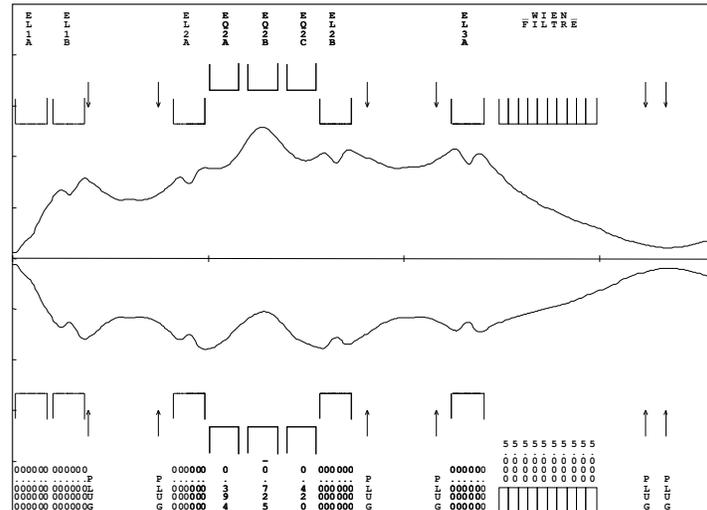
**Figure 13: TRANSPORT simulation of the three plug solution. Above: vertical beam envelope. Below: horizontal beam envelope. The radius of the Einzel lenses amounts to 4.0 cm, the one of the electrostatic quadrupoles to 5.0 cm.**
