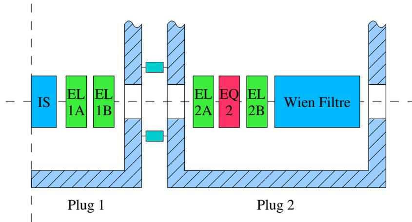
**Figure 14: Two plug option with focal point compensation. The third plug has been cancelled by reducing the quadrupole triplet to a single quadrupole and shifting the Wien filter into the second plug.**
