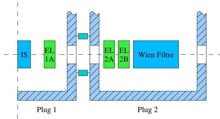
**Figure 16: Two plug solution without focal point compensation. Only one Einzel lens for beam extraction is placed in the first plug, another two for beam capture and the generation of a focus behind the Wien filter in the second one.**
