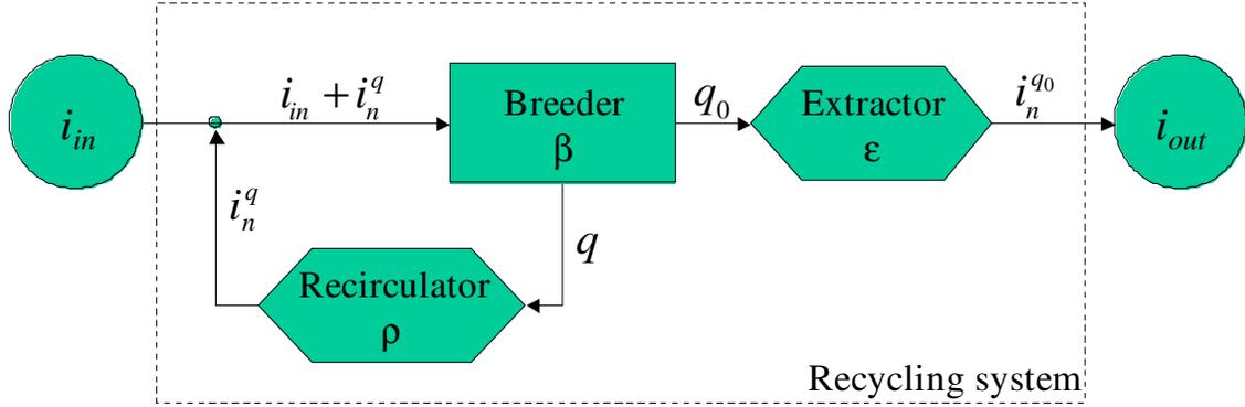
**Figure 27: Flow chart of an ion recycling system with charge breeder, extractor and recirculator.**
