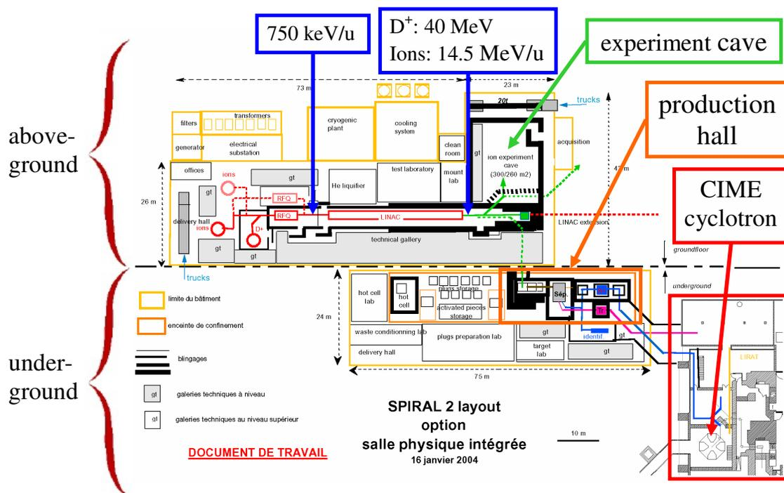
**Figure 1: Layout of the SPIRAL 2 facility. Top: floor plan of the ground floor. Bottom: floor plan of the underground level. The lower right region marked by the red rectangular belongs to the already existing SPIRAL facility.**
