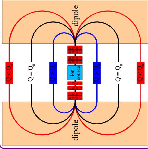
Fig.: Racetrack shaped ion recirculator.
