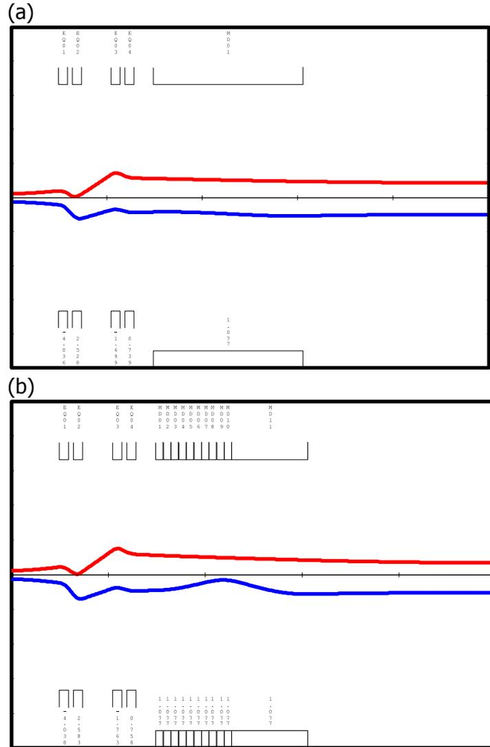
**Figure 30: Beam envelopes of optics 2 for one symmetry element calculated with Graphic TRANSPORT in 2<sup>nd</sup> order without space charge (a) and in 1<sup>st</sup> order for a beam intensity of  $I = 1.0$  mA (b).**
