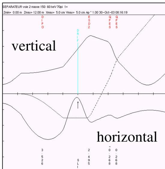
Figure 4: Beam optics of the BRAMA solution.
