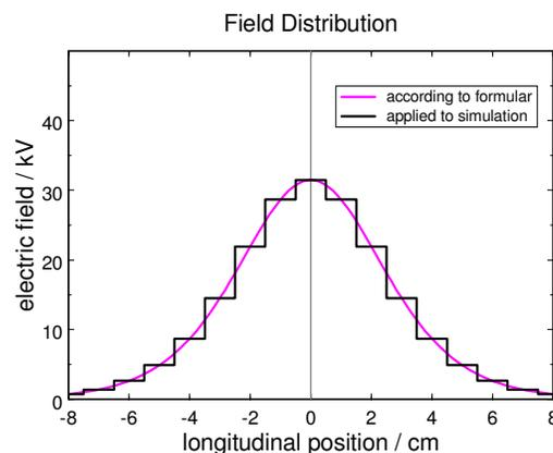
**Figure 12: Longitudinal field distribution of an Einzel lens (magenta, see Appendix 9.2) approximated by a step function (black) for 100 kV supply voltage, 4 cm radius and a length of the inner tube of 1 cm.**
