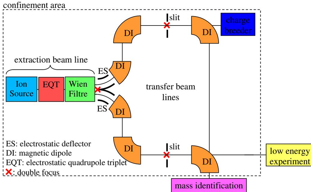
Figure 8: General layout of the Wien filter solution.
