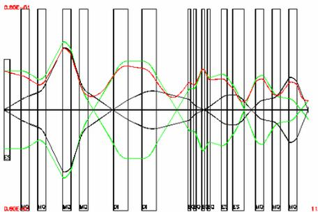
**Figure 24: Vertical beam optics of beam line B. Black: initially point like rays. Green: initially parallel rays. Red: beam envelope.**
