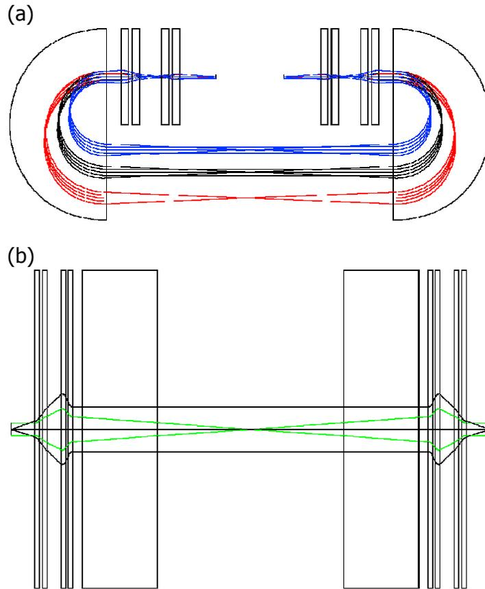
**Figure 29: Optics 1 calculated with COSY in 3<sup>rd</sup> order. (a): Horizontal 2D-illustration for  $Q = 16 e$  (red),  $Q = 20 e$  (black) and  $Q = 24 e$  (blue). (b): Vertical rays of the reference charge  $Q_0 = 20 e$  (black, green).**
