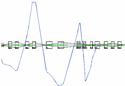
**Figure 25: Dispersion (trajectory of particle with  $\Delta p/p = 1$ ) in beam line B. With the presented setup the initial beam dispersion which depends on the mass separation of the Wien filter can be compensated.**
