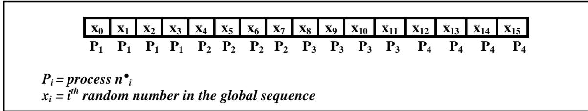
Fig.2. The Sequence Splitting method (with 4 parallel processes)
