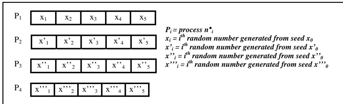
Fig.3. The Independent Sequences method (with 4 parallel processes)
