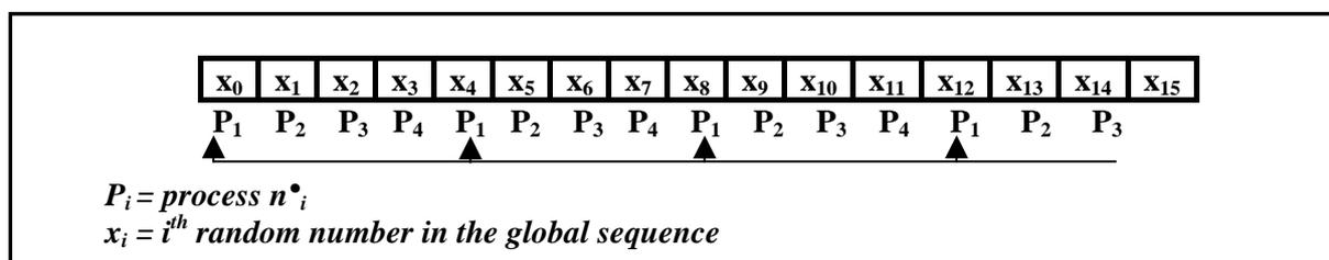
Fig.1. The Leap Frog method (with 4 parallel processes)
