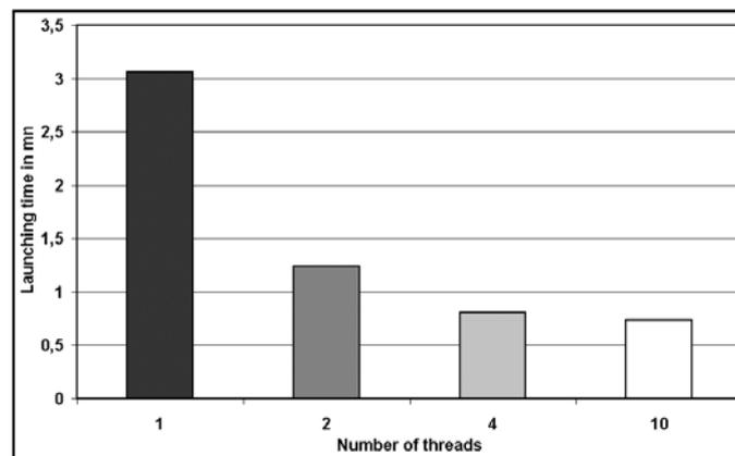
Fig.8. Influence of the number of threads in a parallel launchings
