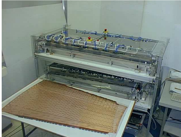
Figure 22: View of the flat test benches. The top part is used to test A and B electrodes, the bottom part is used for C and D electrodes. The electrode just about to be tested is a D electrode.
