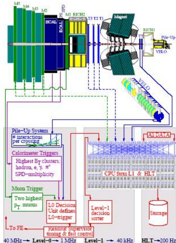
Figure 1. Overview of the LHCb trigger system [1], in parallel with the LHCb detector. Different steps are described with links to the concerned part(s) of the detector.
