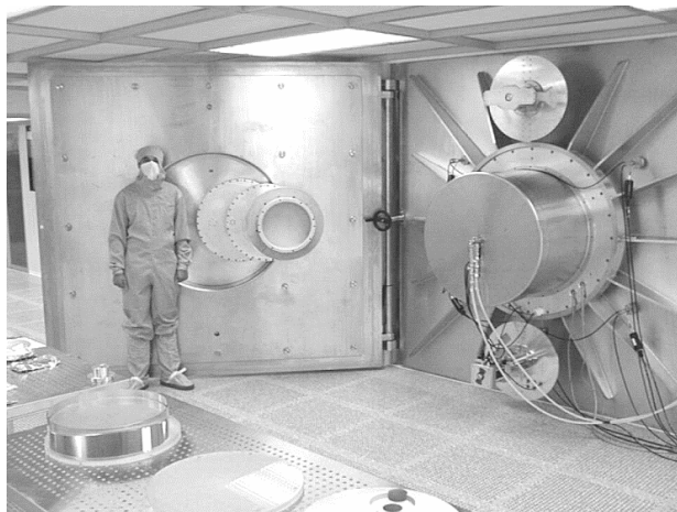
Pictures 1 and 2: IBS deposition system
