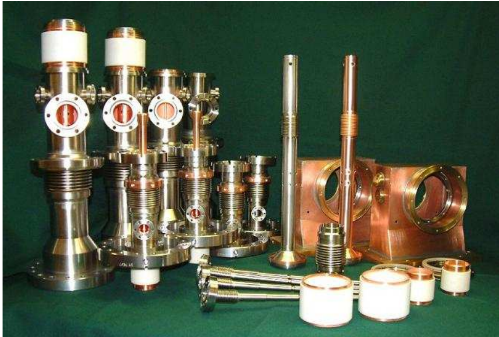
Figure 2. Various coupler parts including warm and cold assemblies, ceramic windows, wave-guide transitions and bellows.
