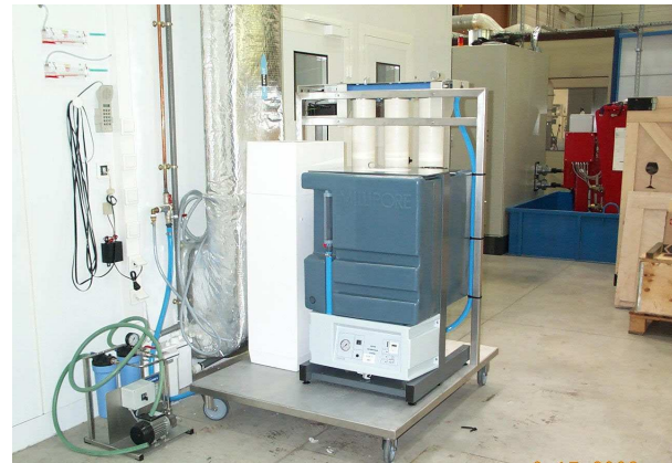
Figure 4. Ultra-pure water production system.
