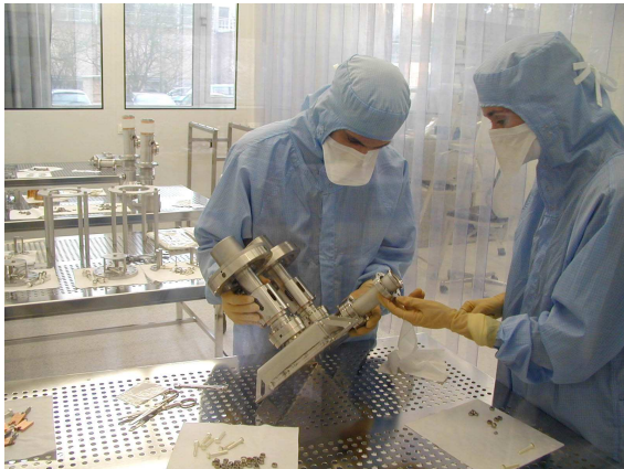
Figure 5. Assembly of cold coupler parts in class 10 clean room
