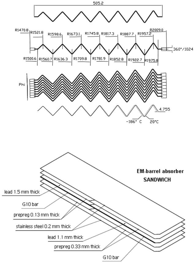
Fig. 3. The upper figure shows the absorber profile and a sketch of a stack of 5 absorbers. The lower figure shows the piling up of the absorber sandwich with the 2 lead thicknesses, before folding the absorber in an accordion shape.
