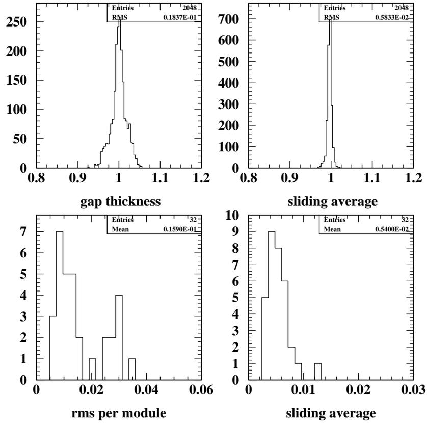
Fig. 17. The top left plot shows the normalized gap thickness deduced from the gap capacity measurements. The top right plot shows the same distribution using a sliding average over 5 consecutive gaps, quantity used to determine the contribution to the constant term. The bottom plots present the rms of the normalized gap thickness for each module.
