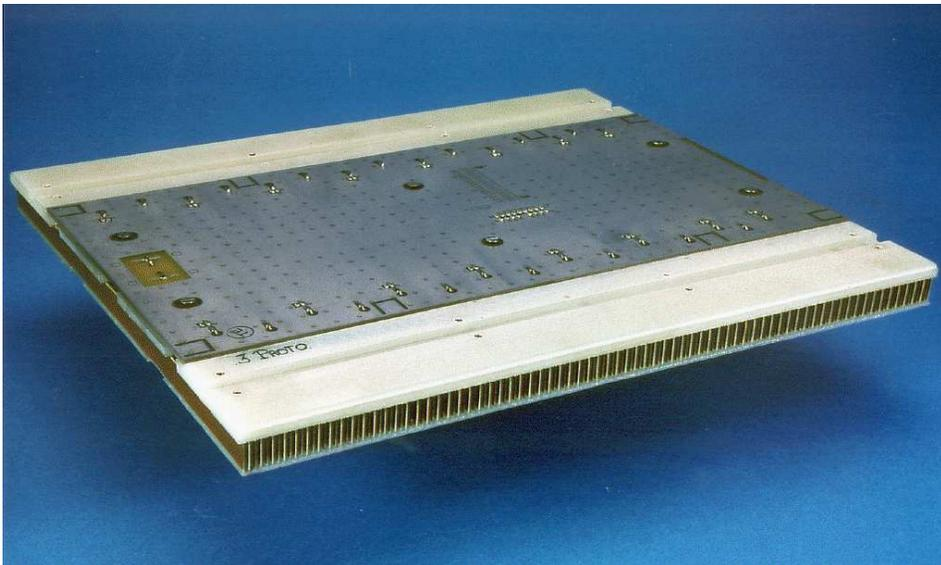
Fig. 9. A presampler module with its motherboard.
