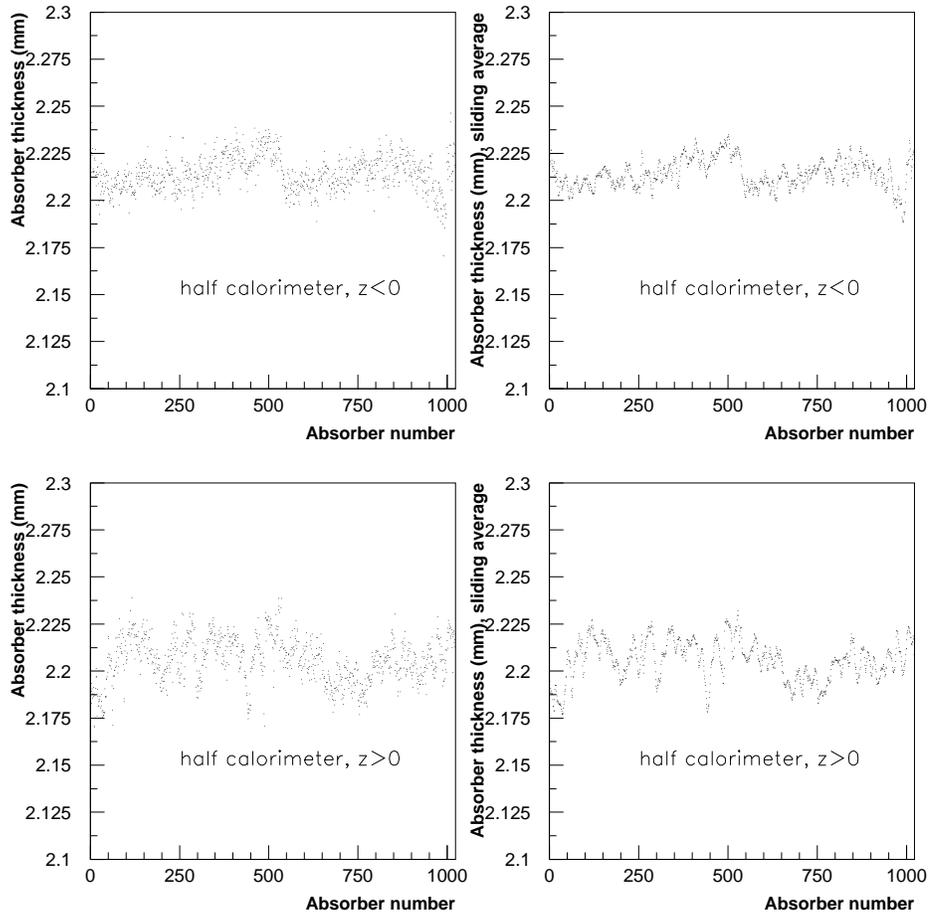
Fig. 12. Distribution of the absorber mean thickness (left plots), and of the thickness averaged over 5 consecutive absorbers (right plots) versus  $\phi$  for the 2 half calorimeters. The stability of the production chain is at the level of 1%.
