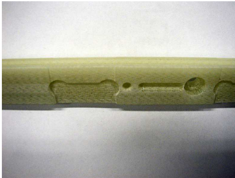
Fig. 4. G10 bar: transverse view drawing showing the 2\pi/1024 angle and picture of a bar section (10 cm long) showing holes for dowel pins and cut-outs for connectors.
