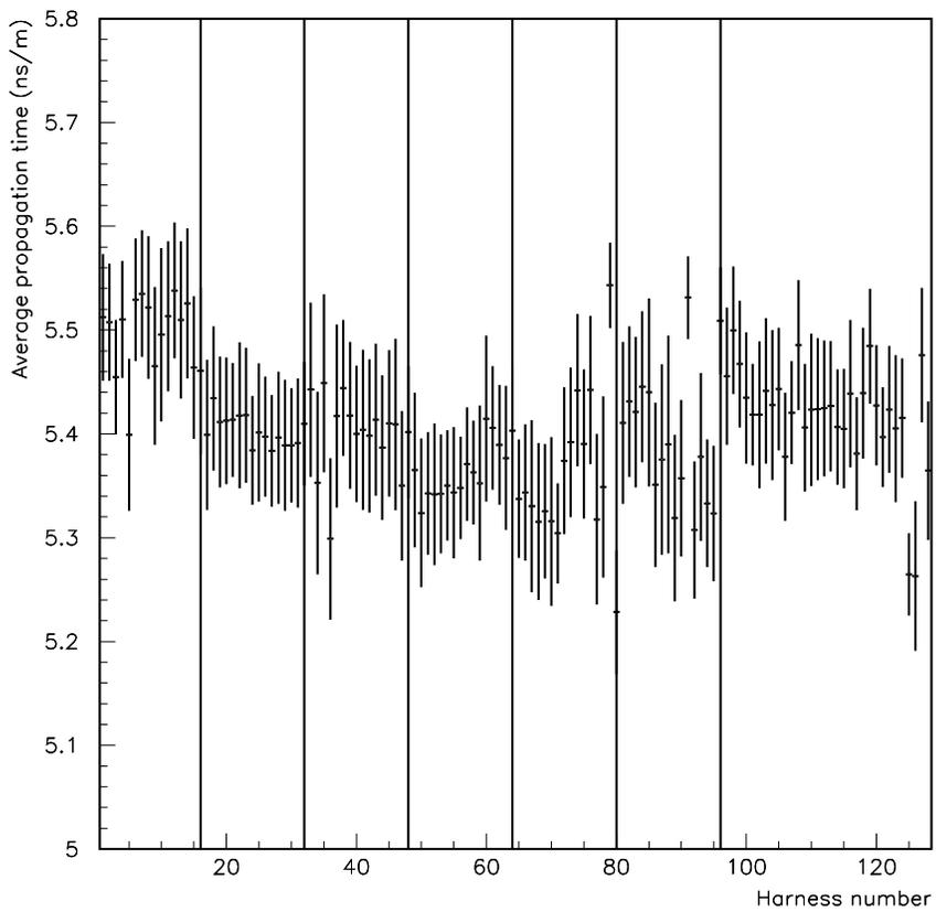
Fig. 19. Average and rms propagation time (per meter) of 4m long 64-channel harnesses equipping the barrel from  $\eta = 0$  to  $\eta = 0.2$ . The vertical lines separate different batches from the manufacturer.
