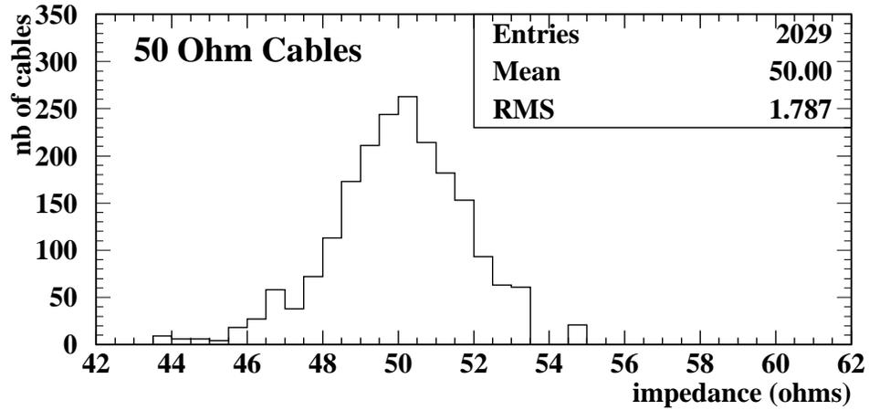
Fig. 18. Distribution of the impedances of the 25  $\Omega$  and the 50  $\Omega$  cables. This measurement was performed by cutting a 70 cm piece at the end of each 200 m long cable coil.
