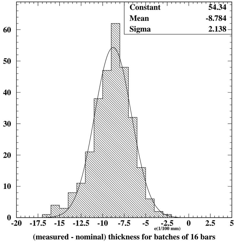
Fig. 14. Difference between actual and nominal thickness for 30 batches of 16 external bars and 30 batches of 16 internal bars. On average the batches are a bit too thin (average -0.09 mm, rms 0.02 mm).
