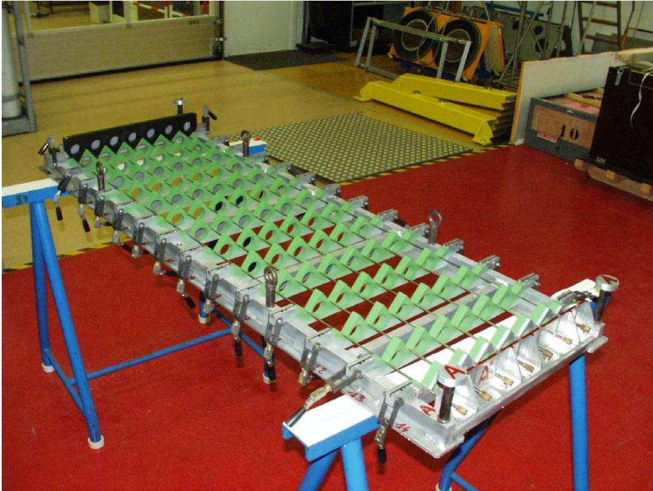
Fig. 16. Tooling used to produce a spacer.
