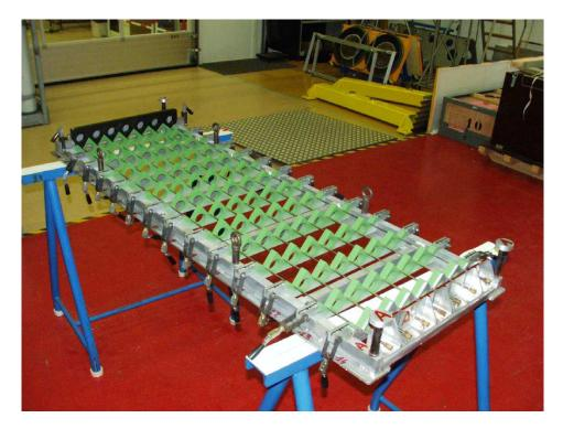
Fig. 16. Tooling used to produce a spacer.
