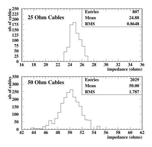
Fig. 18. Distribution of the impedances of the  $25 \Omega$  and the  $50 \Omega$  cables. This measurement was performed by cutting a 70 cm piece at the end of each 200 m long cable coil.
