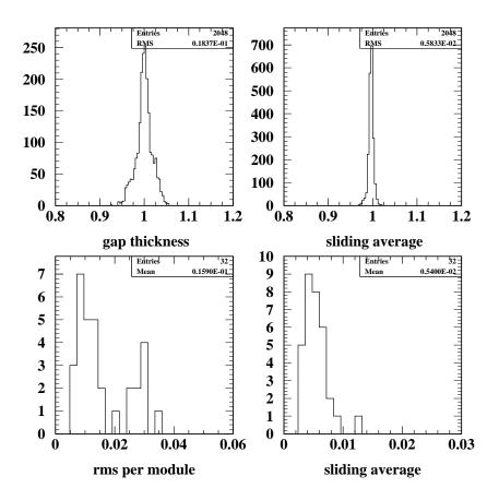
Fig. 17. The top left plot shows the normalized gap thickness deduced from the gap capacity mesurements. The top right plot shows the same distribution using a sliding average over 5 consecutive gaps, quantity used to determine the contribution to the constant term. The bottom plots present the rms of the normalized gap thickness for each module.
