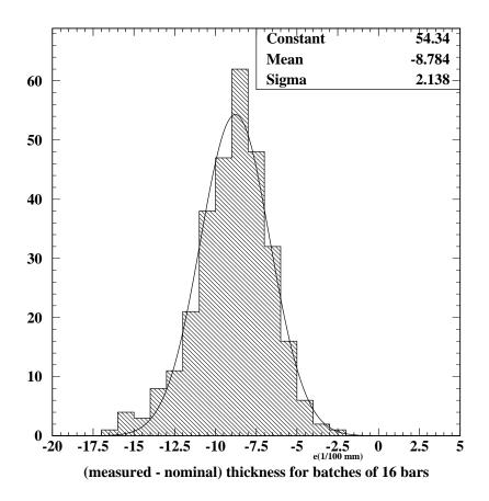
Fig. 14. Difference between actual and nominal thickness for 30 batches of 16 external bars and 30 batches of 16 internal bars. On average the batches are a bit too thin (average -0.09 mm, rms 0.02 mm).
