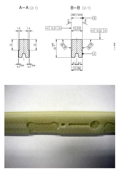
Fig. 4. G10 bar: transverse view drawing showing the  $2\pi/1024$  angle and picture of a bar section (10 cm long) showing holes for dowel pins and cut-outs for connectors.
