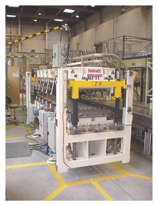
Fig. 11. Picture of the heating press where the absorber is placed for curing after folding.
