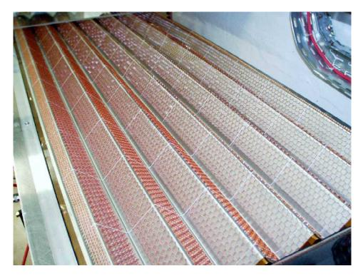
Fig. 8. One spacer resting on one absorber.
