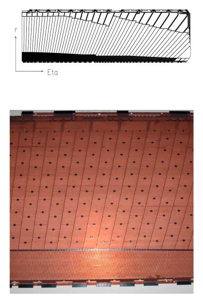
Fig. 7. Upper part: etched pattern, before folding, on A+B electrodes signal layer. Lower part: picture of a section, about 50 cm long, of an A electrode, before folding, showing the etched pattern of the HT layer where the resistive silk-screened pads of carbon-loaded epoxy ink can easily be seen. (The copper strips between connectors have not yet been removed.)
