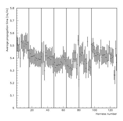
Fig. 19. Average and rms propagation time (per meter) of 4m long 64-channel harnesses equipping the barrel from  $\eta = 0$  to  $\eta = 0.2$ . The vertical lines separate different batches from the manufacturer.
