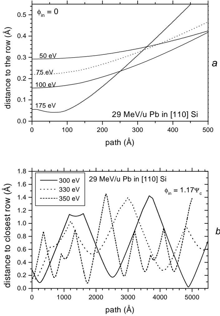
Figure 2: Trajectories of 20 MeV/u  $\text{Pb}^{56+}$  along [110] silicon atomic rows. *a*) Ion trajectories for various transverse energies (beam aligned with [110] axis). *b*) Ion trajectories for a tilted beam and various transverse energies.
