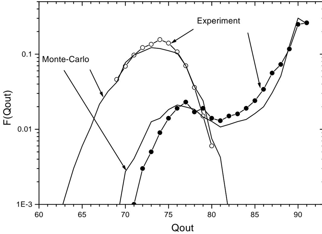
Figure 8: 20 MeV/u  $U^{91+}$  ions incident on a  $11.7\mu m$  Si crystal. Charge distributions for [110] axial (full circles) and random (open circles) geometries, and associated Monte-Carlo calculated curves.
