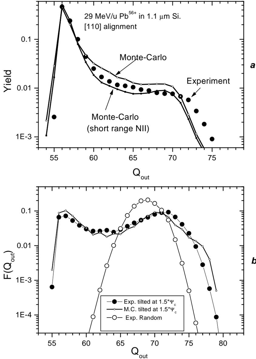
Figure 4: Measured charge state distributions for 29 MeV/u Pb<sup>56+</sup> ions channeled in a 1.1  $\mu\text{m}$  thick silicon crystal and corresponding Monte-Carlo calculated distributions. ) [110] alignment for two different impact parameter distributions for NII. ) For a tilted angle  $1.5 \times \Psi_c$ ; the Omidvar [15] probabilities for cascading per unit times (see appendix A) were divided by a factor 5. The distribution corresponding to a random orientation is also represented.
