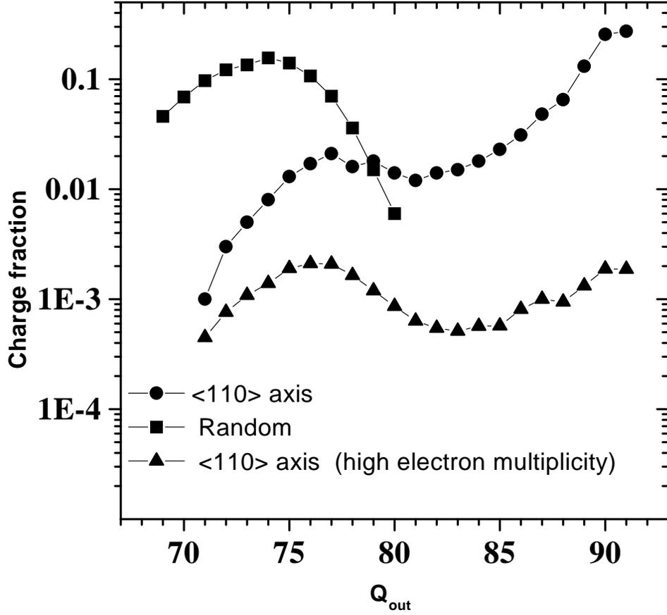
Figure 6: Charge distributions for 20 MeV/u incident  $U^{91+}$  ions after transmission through a  $11.7\mu m$  silicon crystal : random incidence ( $\blacksquare$ ),  $[110]$  alignment ( $\bullet$ ), (these two distributions are normalized to 1);  $[110]$  alignment and high electron multiplicity ( $\blacktriangle$ ) (see text); this last distribution is normalized to 0.02 which is the corresponding ion fraction.
