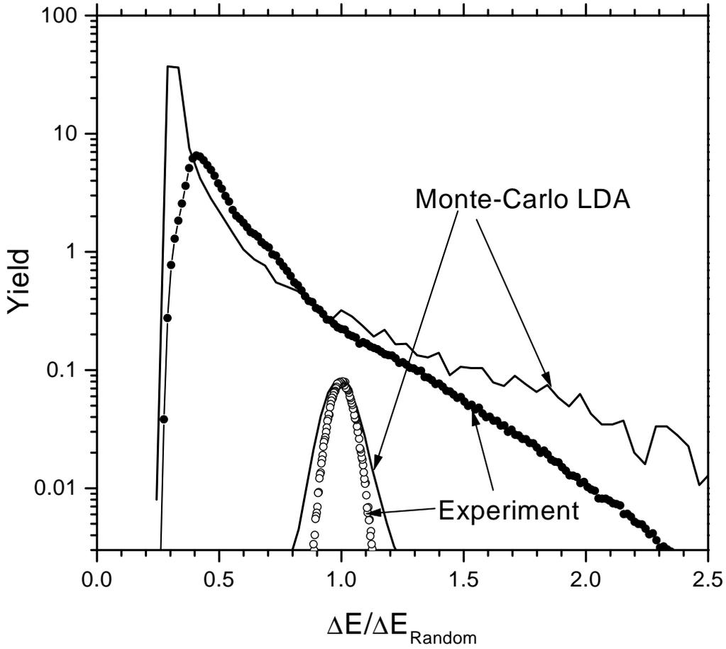
Figure 5: Energy loss spectra for 29 MeV/u  $\text{Pb}^{56+}$  ions channeled along the [110] axis of a  $1.1\mu\text{m}$  thick silicon crystal and for random geometry. Energy loss is normalized to the mean random energy loss for  $Q_{\text{out}}=68$ . Black and open circles: experimental spectra, respectively for aligned and random geometries. Solid lines: Spectra calculated by Monte-Carlo.
