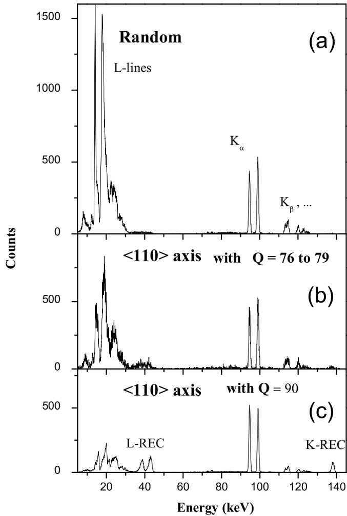
Figure 7: 20  $MeV/u$   $U^{91+}$  ions incident on a  $11.7\mu m$  Si crystal. X-ray recorded at  $90^\circ$  to the beam : for random conditions (a), for  $[110]$  alignment and ions transmitted with charge states 76 to 79 (b), and with charge 90 (c). The spectra are normalized to the same number of transmitted ions with the given selection.
