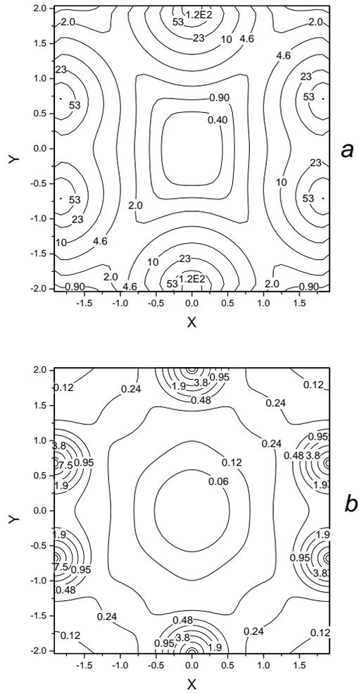
Figure 1: *a)* Potential in Si [110] channel for a unit charge, averaged along the [110] direction (labelled in eV). *b)* Electronic density averaged along the [110] direction (labelled in electrons per cubic angström)
