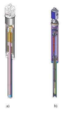
Fig. 1: a) first conceptual design of the target system; b) present conceptual design of the target system.
