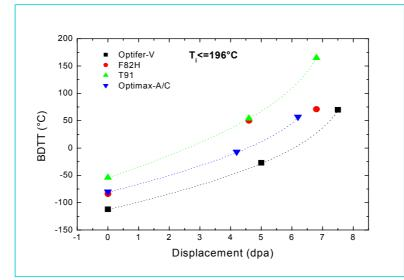
Fig. 5: DBTT vs dpa data obtained on the steels irradiated at SINQ (STIP-I) [4]. The T91 steel exhibit a DBTT of 230  $^{\circ}$ C (temperature corresponding to the hot – standby of the MEGAPIE target) at about 8,6 dpa and 730 appm of He.
