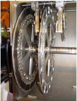
Figure 1: Target chamber with the two wheels bearing 18 Pb or Bi targets and 18 carbon charge equilibration films.
