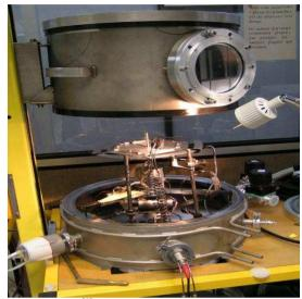
Figure 2: System for evaporating <sup>208</sup>Pb or Bi onto rotating carbon backings.
