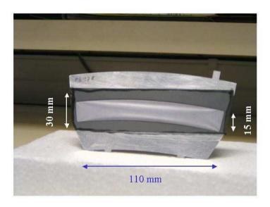
Figure 3: Enriched  $^{208}Pb$  target, 15 mm in height, 100 mm long: C 35  $\mu g/cm^2$  + Pb  $\,350~\mu g/cm^2$  + C 5  $\mu g/cm^2$  .
