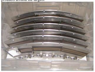
Figure 4: 208 Pb targets on segments of the wheel after irradiation.
