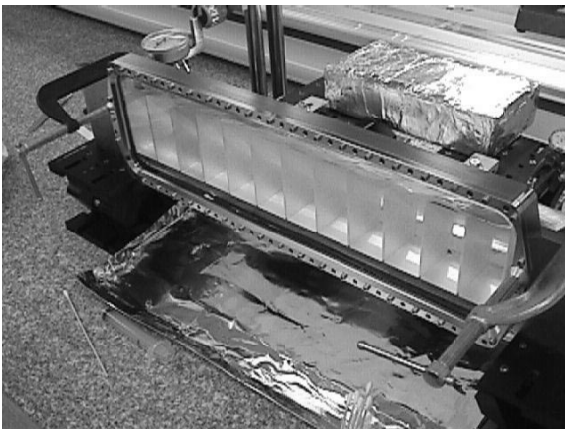
Figure 28. End view of the window of a bar box showing the window-frame, fused-silica window and twelve wedges.
