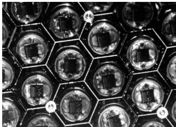
Figure 39. PMTs and rhodium-plated light-catchers in the SOB.
