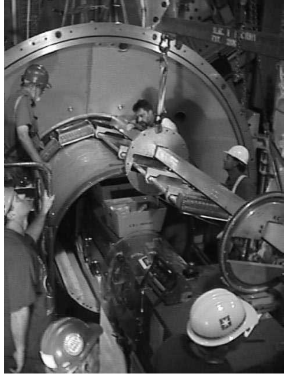
Figure 30. Installation of a bar box into the BABAR detector. Not seen in the figure is the cantilevered support arm which supports the installation fixture above the accelerator components.
