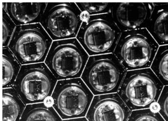
Figure 39. PMTs and rhodium-plated light-catchers in the SOB.
