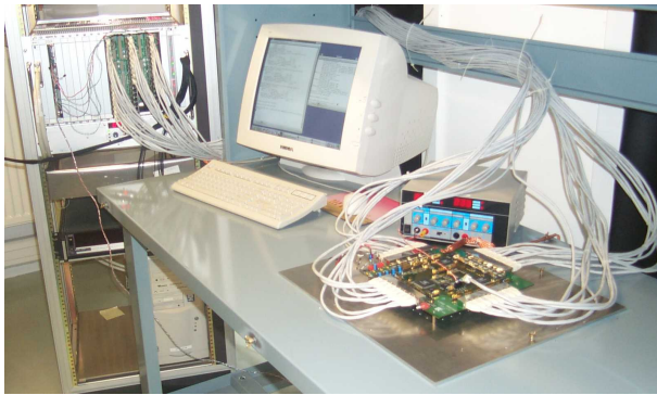
Figure 5.2: L0DU prototype and its test set-up
