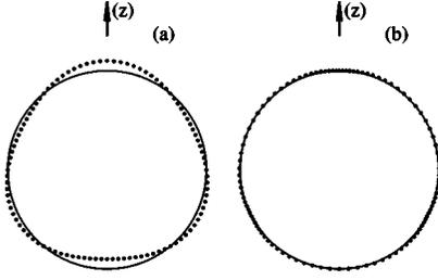
FIG. 1. Radial (a) and tangent (b) distortions of a spherical shell having the same symmetry. The corresponding displacement fields  $Y_{30}$  (a) and  $Z_{30}$  (b) span  $D_3[-1]$  representation of the  $O_3$  symmetry group. The vertical direction coincides with the  $z$  axis.
