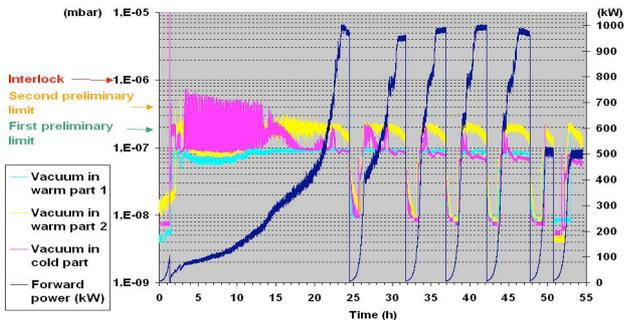
Figure 3: Forward power monitoring based on vacuum levels.
