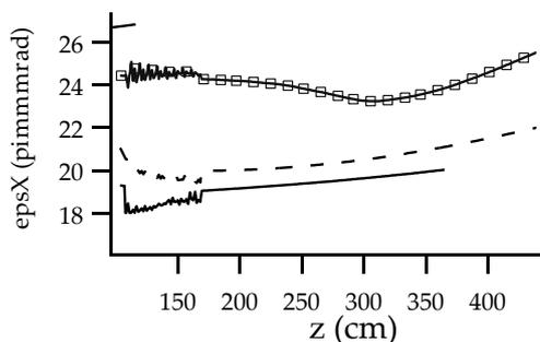
Figure 7: Emittance as a function of distance for several kinds of magnetic field. The SLAC section is located at  $z = 107$  cm and has a length of 63 cm and a gradient of 30 MV/m. The position of the coils is variable; square points, coil at  $z = 15$  cm and  $B_z = 0.21$  T; dashed line, 2 coils at  $z = 10$  cm and 20 cm and  $B_z = 0.23$  T; plain line, 2 coils at  $z = 2$  cm and 10 cm and  $B_z = 0.25$  T.
