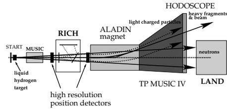
Fig. 1. Schematic SPALADIN experimental set-up. Distance between  $^1\text{H}_2$  target and hodoscope is 8 m roughly.
