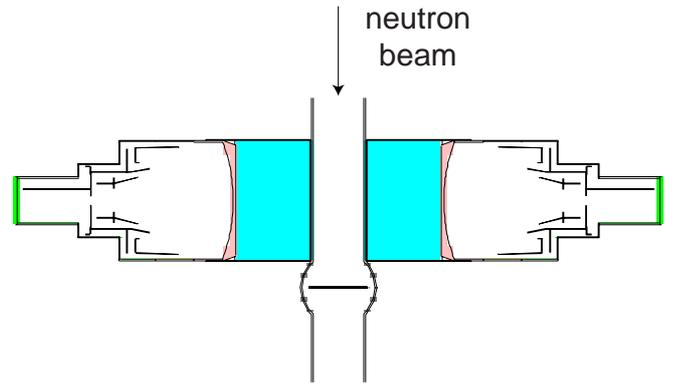
FIG. 1: (Color online) A schematic view of the horizontal plane of the detectors and sample geometry in the  $^{232}\text{Th}(n,\gamma)$  measurement. Neutrons going through the 5.8 cm inner diameter beam tube are incident on the sample placed in the beam. Two  $\text{C}_6\text{D}_6$  detectors, each one consisting of a scintillator cell of 12.7 cm in diameter and 7.62 cm high coupled to a photomultiplier, are placed 9.2 cm upstream with respect to the sample center.
