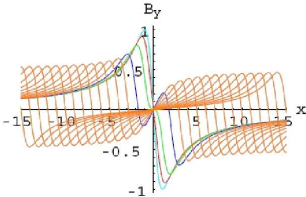
Figure 3: Pairs contributions to vertical component of the magnetic field with  $n < 1$  for light blue and red curves,  $n = 1$  for the green curve, and  $n > 1$  for the dark blue ( $n = 2$ ) and orange curves.
