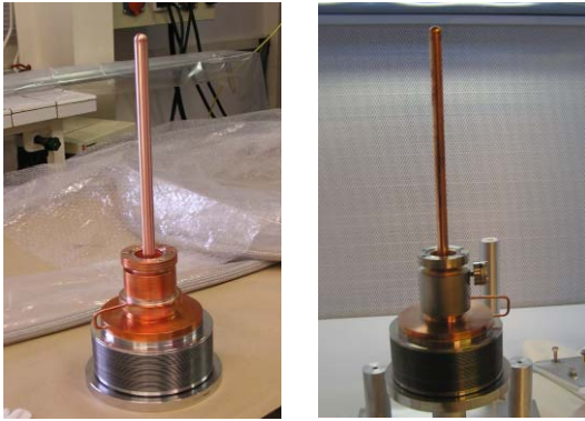
Figure 3: Prototype with disc window (left) and cylindrical window (right).
