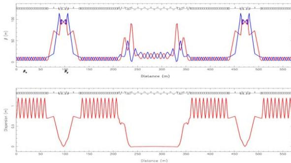
Figure 4: Optical functions for triangle lattice (long production straights are not shown).
