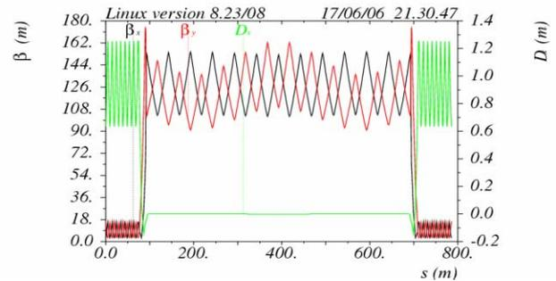
Figure 5: Optical functions: horizontal (black) and vertical (red) and dispersion (green) for  $1/2$  the racetrack design. The production straight is shown in the center.
