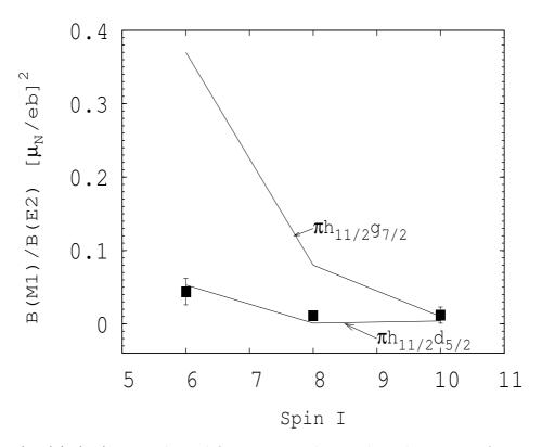
FIG. 12: B(M1)/B(E2) ratios derived from measured  $\gamma$ -ray branching ratios for Bands 3 and 4 and calculated values for the  $\pi h_{11/2} d_{5/2}$  and  $\pi h_{11/2} g_{7/2}$  configurations.
