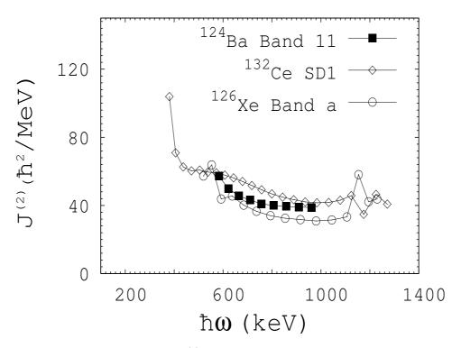
FIG. 15: Dynamic moment of inertia,  $\mathcal{J}^{(2)}$ , for Band 11 in  $^{124}$ Ba as well as for similar bnds in  $^{132}$ Ce [48] and  $^{126}$ Xe [49], as a function of rotational frequency.
