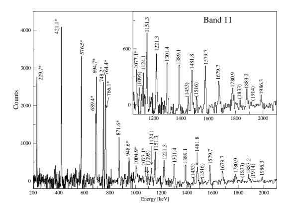
FIG. 4: Summed triple-gated coincidence spectrum of Band 11. The spectrum was produced by setting one gate on transitions (229.7 to 1077 keV) of Band 1 and two gates on transitions (1124.1 to 1986.3 keV) of Band 11. The asterisks mark peaks of Band 1. The energies in parentheses correspond to transitions which are observed in coincidence but could not be placed in the level scheme.
