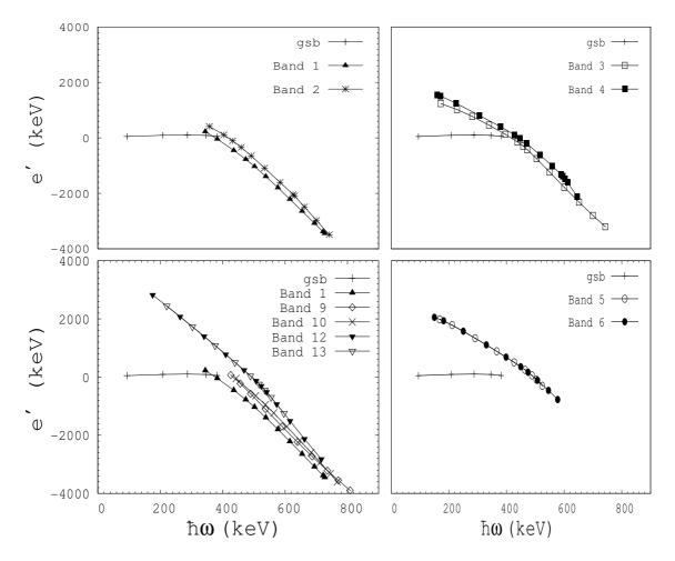
FIG. 10: Experimental routhians, e', as a function of rotational frequency. A reference core with Harris parameters  $\mathcal{J}_{\circ} = 17 \; \hbar^2 \mathrm{MeV}^{-1}$  and  $\mathcal{J}_{1} = 26 \; \hbar^4 \mathrm{MeV}^{-3}$  has been subtracted.
