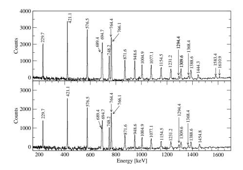
FIG. 2: Summed triple-gated  $\gamma$ -ray coincidence spectra of Band 1. The upper spectrum was produced by setting two gates on transitions (689.4 to 1444.3 keV) of Band 1 and one gate on the 1454.8 keV transition. The lower spectrum was obtained by setting two gates on transitions (689.4 to 1454.8 keV) of Band 1 and one gate on the 1444.3 keV transition.
